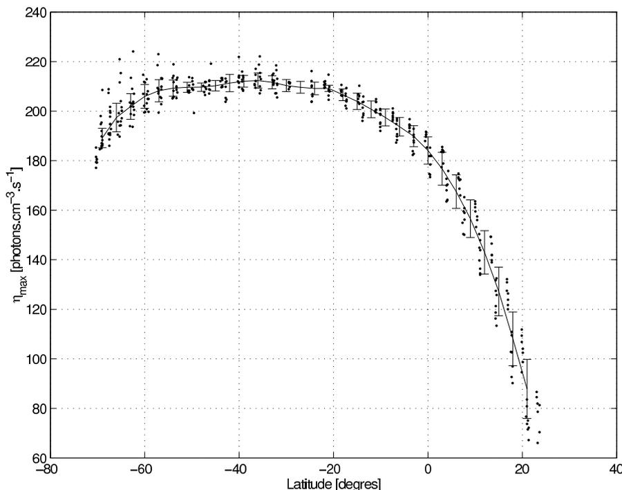
**Fig. 6.** WINDII data of the oxygen red emission measured on 1 April 1992 ( $A_p=13$ ,  $f_{10.7}=191.4$ ). Dots represent the WINDII 630.0 nm VER data plotted versus latitude, and the line represents the corresponding zonal average. Error bars indicate the standard deviation.
