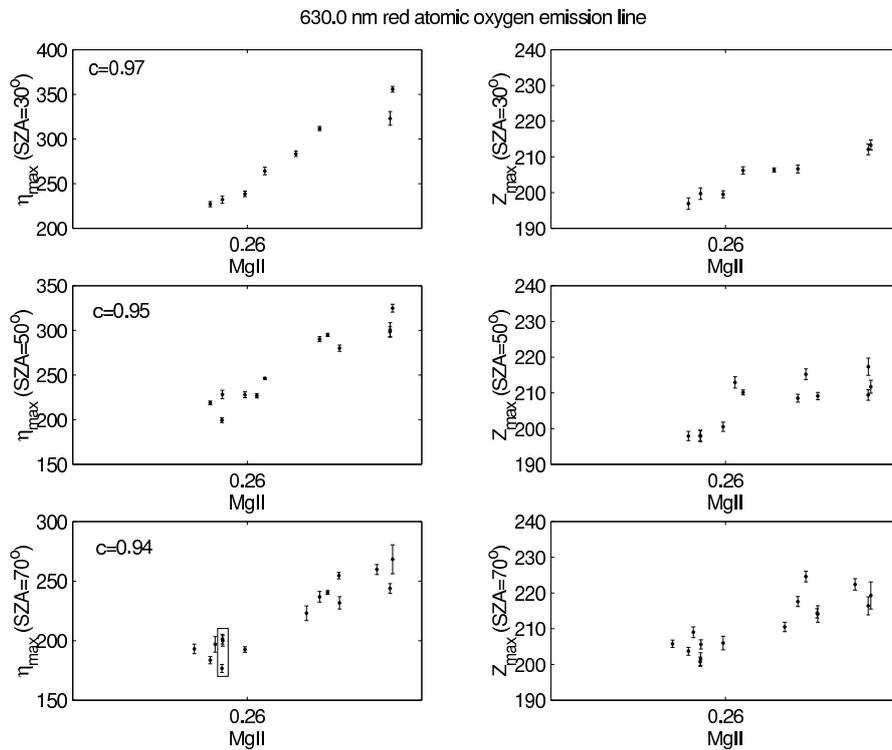
**Fig. 12.** WINDII measurements of the 630.0 nm volume emission rates and maximum emission altitudes for quiet geomagnetic days ( $A_p \leq 10$ ), from 1992 to 1995. Data are plotted versus the  $MgII$  index, and error bars correspond to the standard deviation.
