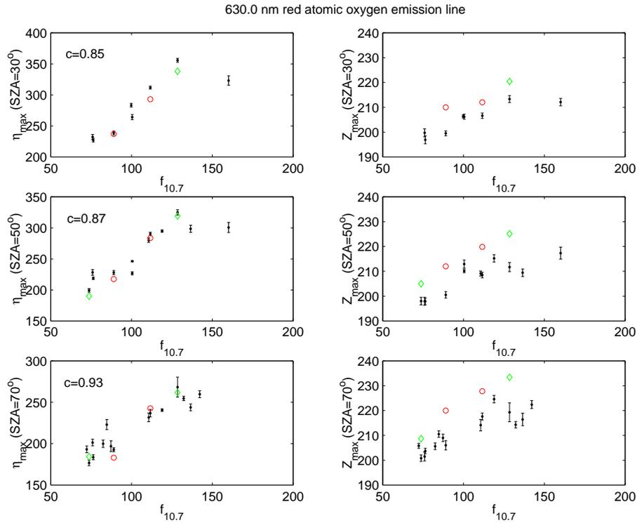
**Fig. 11.** WINDII measurements of the 630.0 nm volume emission rates and maximum emission altitudes for quiet geomagnetic days ( $A_p \leq 10$ ), from 1992 to 1995. Data are plotted versus the  $f_{10.7}$  index, and error bars correspond to the standard deviation. Diamonds correspond to the TRANSCAR simulation results presented in Sect. 4.1.1, and circles are simulations results for intermediate solar activity.
