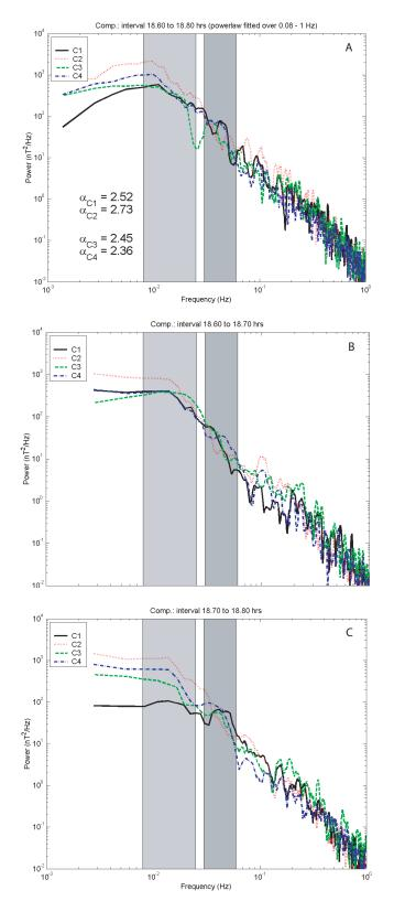
**Fig. 9.** The power spectra for the 12 August data. Panel (a): The power spectra for all spacecraft for the total interval 18:38-18:46 UT. Panel (b): The power spectra for all spacecraft during the first half of the interval, with C3 in the same region as C1/2/4. Panel (c): The power spectra for all spacecraft during the second half of the interval, with C3 at the opposite side of the neutral sheet with respect to C1/2/4. For clarity the fitted power laws have not been plotted in the panels.
