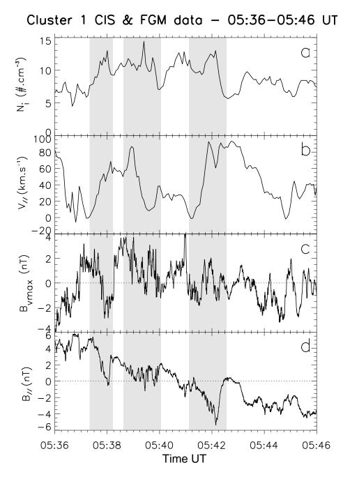
Fig. 8. Plasma injection events observed at Cluster. (a) Ion density. (b) Ion parallel velocity. (c) Perpendicular component and (d) parallel component of the magnetic field (see text).
