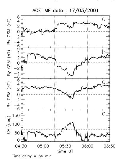
Fig. 3. Interplanetary magnetic field (IMF) from the ACE spacecraft on 17 March 2001 for the period 04:30–06:30 UT. Data are lagged by 86 min to take into account the delay from the spacecraft to the ionosphere. Panels (a), (b) and (c) show, respectively, the IMF  $B_x$ ,  $B_y$  and  $B_z$  components in GSM coordinates. Panel (d) shows the IMF clock angle.
