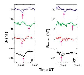
**Fig. 9.** Cluster magnetic field variations around the burst at 05:42:30 UT (Burst 3 of Fig. 10). (a) Parallel component. (b) Perpendicular component in the direction of maximum variance. The colour identification of the spacecraft is the same as for Fig. 1. Arrows indicate the time of observation of a similar variation at each spacecraft.
