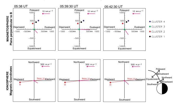
**Fig. 10.** Phase velocity vector of three injections events determined from Cluster FGM and associated with flow bursts observed by Super-DARN. Top: at the Cluster location in the plane perpendicular to the magnetic field and in GSE coordinates with the relative position of the four spacecraft. Bottom: projection of the Cluster velocity into the ionosphere in AACGM coordinates. The direction of beam 14 of the Hankasalmi radar at the Cluster footprint is also shown.
