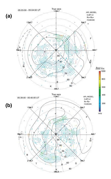
**Fig. 11.** Global convection velocity maps deduced from SuperDARN data of the Northern Hemisphere radars according to the method of Ruohoniemi and Baker (1998), at two selected times for (a) IMF  $B_y > 0$  and (b) IMF  $B_y < 0$ . The black solid lines represent the equipotential contours and the colour dots represent the grid points where the convection vectors are determined.
