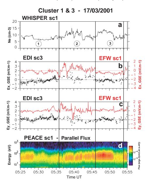
**Fig. 5.** WHISPER, EFW, EDI and PEACE data for the period 05:25–05:55 UT, with three sub-intervals. (a) WHISPER (SC1) electron density. (b) and (c) *x* and *y* components of the electric field in GSE coordinates for EFW (SC1) (red line) and EDI (SC3) (black crosses). The offset of the EFW data has been corrected. (d) PEACE (SC1) energy-time spectrogram of precipitating electrons, in the  $0 - 20^{\circ}$  pitch angle range (Calibration 1.5).
