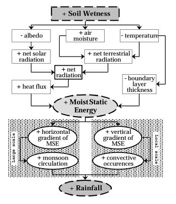
**Fig. 8.** Schematic diagram of the basic soil moisture – rainfall feedback in the boundary layer (adapted from Emanuel (1995), Eltahir and Gong (1996), Zheng and Eltahir (1998), and our results).
