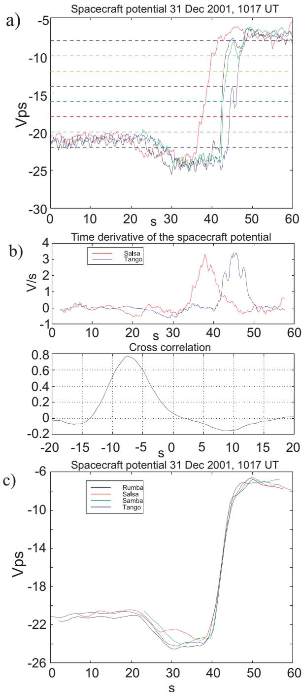
**Fig. 4.** (a) The parameter  $v_{ps}$  for all four satellites, with a few specific potentials indicated, (b) the derivative of this potential for two satellites and the corresponding cross-correlation, (c) the low pass filtered potentials shifted in time to overlap. In this lower panel 10 s correspond to about 1000 km.
