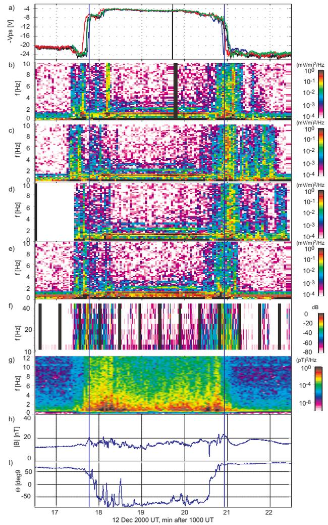
**Fig. 3.** Cluster observations from 31 December 2000. This display corresponds to the latter part of Fig. 2, and the upper seven panels are similar to that figure. (Note the data gap during the first minute in panel (d)). Panels (h) and (i) show the magnitude of the magnetic field from FGM on satellite 4, and the elevation angle of this field (so that  $90^\circ$  corresponds to a strictly northward field), respectively.
