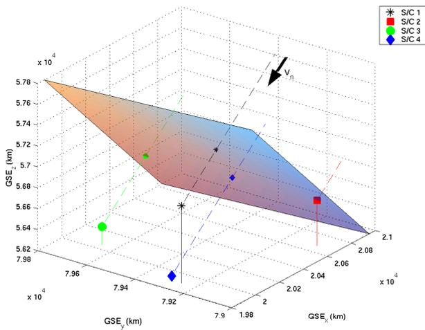
**Fig. 5.** A sketch of the location of the Cluster satellites and the orientation of the magnetopause during the magnetopause crossing on 31 December 2000, near 10:17 UT. Satellites 1 to 4 are indicated by black, red green and blue, respectively.
