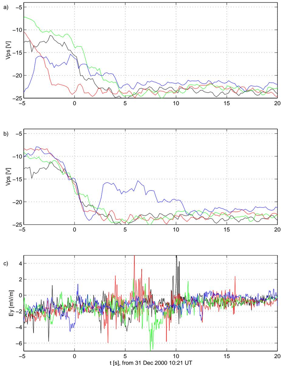
**Fig. 8.** (a) The potential  $v_{pS}$  from 10:21:00 UT on 31 December 2000, for all four Cluster satellites (1: black; 2: red; 3: green; 4: blue), (b) The same signals, but shifted in time to correspond to a common moving magnetopause frame. (c) The  $E_y$  component of the electric field for all four satellites, shifted as in panel (b).
