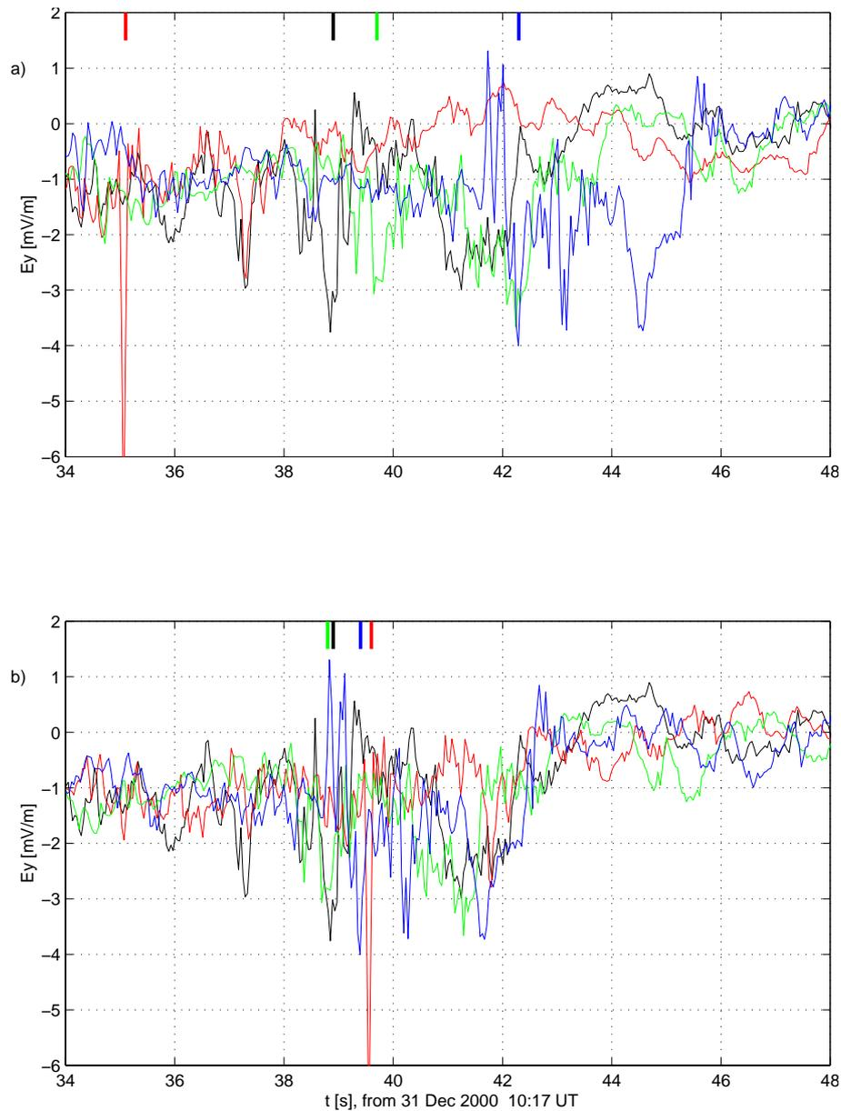
**Fig. 7.** (a) The  $E_y$  component of the electric field from 10:17:00 UT on 31 Decemeber 2000, for all four Cluster satellites (1:black; 2:red; 3:green; 4:blue), (b) The same signals, but shifted in time to correspond to a common moving magnetopause frame.
