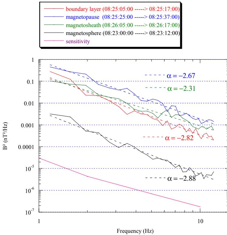
**Fig. 5.** Comparison of the spectra in the regions adjacent to the magnetopause on spacecraft 2. For reference, the sensitivity of the instrument is plotted showing that the fluctuations are much higher, even in the magnetosphere.
