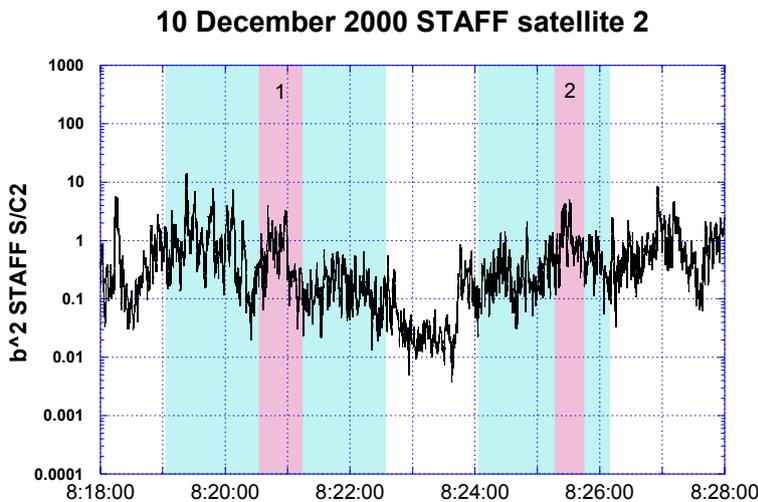
**Fig. 4.** Power of the fluctuations from the STAFF experiment on spacecraft 2, integrated between 0.1 and 10 Hz.
