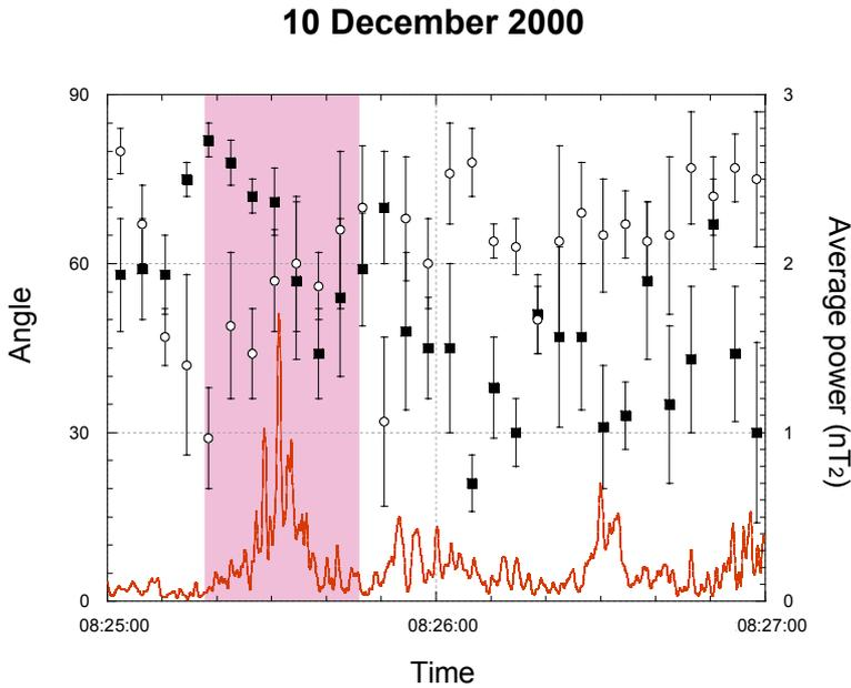
**Fig. 6.** MVA results for 0.35 Hz fluctuations for crossing 2. The points are the values of the angles between  $B_0$  and the direction of maximum variance ( $\blacksquare$ ) and minimum variances ( $\circ$ ) averaged on the four spacecraft. The error bars are the mean square differences of the four values with this average. The position of the magnetopause is shown by the shaded zone and the average power of the fluctuations is drawn for comparison.
