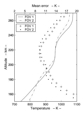
**Fig. 3.** Mean temperature profiles for the two FOVs on day 378. The mean errors are indicated by dots and crosses, and refer to the upper horizontal scale. They are the smallest around the altitude of the maximum of the  $O(^{1}D)$  layer.
