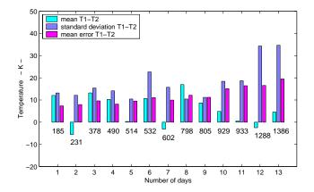
**Fig. 4.** Mean apparent temperature differences between the two FOVs for 13 days, averaged over the tangent altitude range of 180 to 260 km. The standard deviations of the differences and the mean errors are also indicated.
