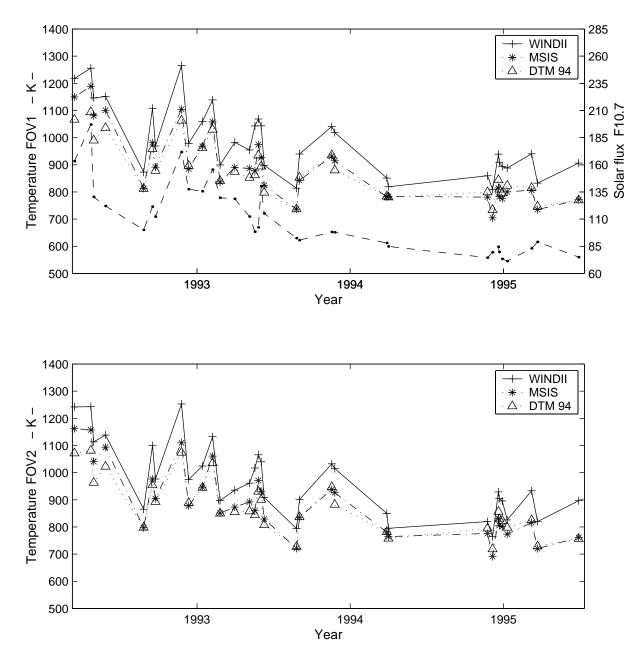
**Fig. 6.** Mean temperatures averaged over the altitude range of 180 to 260 km for 33 quiet days. The upper and lower panels correspond, respectively, to FOV 1 and 2. WINDII data are plotted with the continuous line, while the temperatures obtained from the MSIS-90 and DTM-94 models are, respectively, plotted with the dash-dotted and the dotted lines. The F10.7 cm index (of the previous day) is shown as a dashed line in the upper panel. The corresponding scale is on the right side of the plot.
