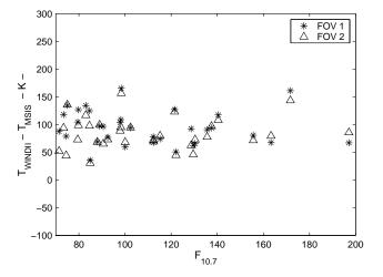
**Fig. 9.** Differences between the mean daily temperatures observed by WINDII and given by the MSIS-90 empirical model for the quiet days as a function of the solar activity.
