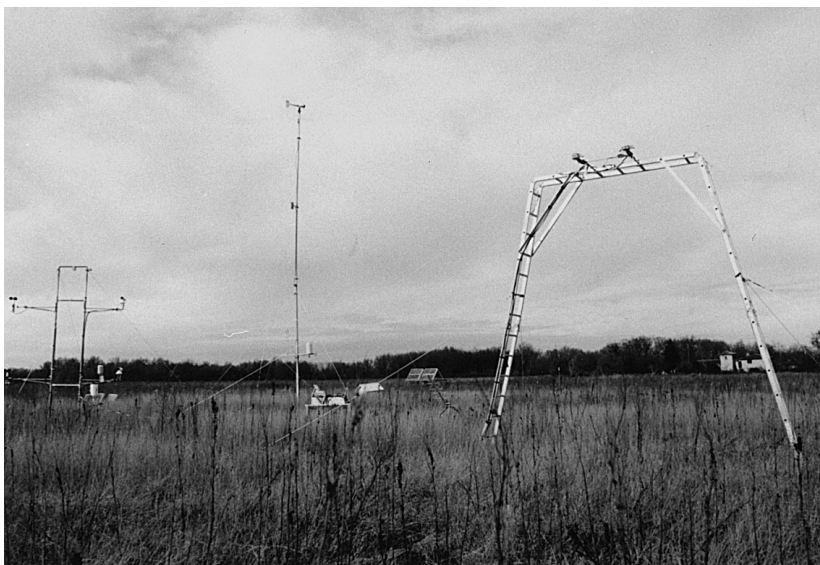
Fig. 1. Photograph of the central part of the MUREX fallow site (at the end of 1996) with some of the instrumentation. From left to right: the two-level SAMER system, the 10-m mast for wind, screen-level temperature and humidity, and IR-temperature, and the scaffolding bearing the radiation sensors
