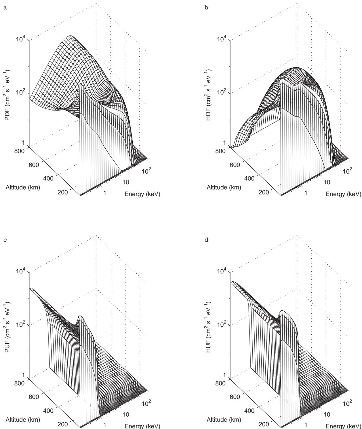
**Fig. 5.** **a** Downward proton flux, **b** downward H atom flux, **c** upward proton flux, and **d** upward H atom flux, as a function of altitude and energy. These fluxes have been integrated over the half pitch angle grid. The upward fluxes result from the effect of collisions
