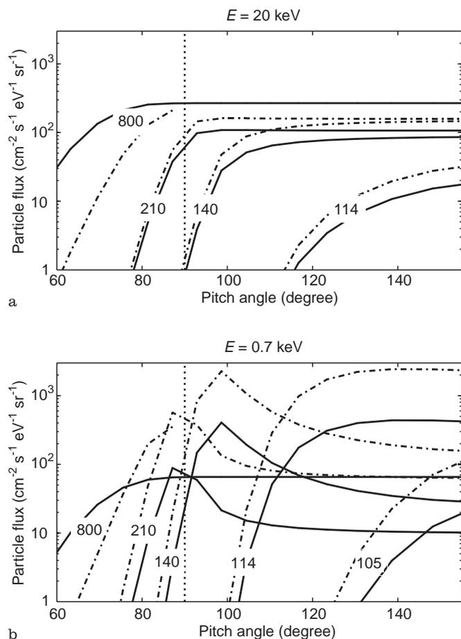
**Fig. 3.** **a** Particle fluxes as a function of pitch angle, for different altitude levels (in km) and for an energy of 20 keV. Proton flux is shown with *solid lines* and H atom flux is plotted with *dashed-dotted lines*. The upward fluxes, related to pitch angles lower than  $90^\circ$ , result from the magnetic mirror force. **b** *idem*, but for an energy of 0.7 keV
