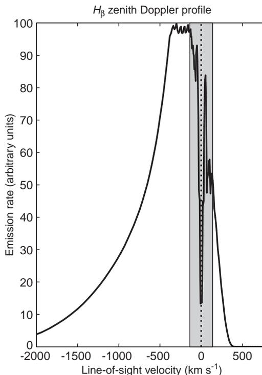
**Fig. 7.** Normalized  $H_{\beta}$  Doppler profiles as a function of line-of-sight velocity, in the magnetic zenith. The *shaded area* represents the part of the profile which can be affected by particles of energy lower than the minimum energy of the computation grid, that is 100 eV. This profile has been obtained from the model including collisional angular redistribution
