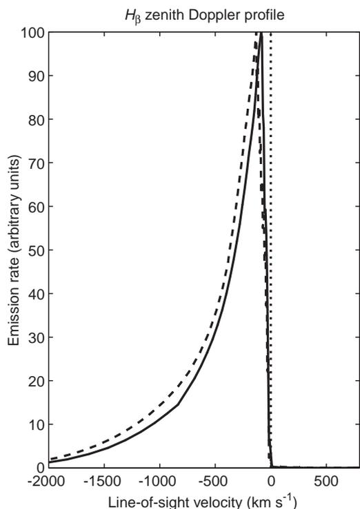
**Fig. 4.** Normalized  $H_\beta$  Doppler profiles as a function of line-of-sight velocity, in the magnetic zenith. The *dashed line* has been computed with a minimum energy of 100 eV, the *solid line* with a minimum energy of 40 eV. Both profiles have been normalized individually. These profiles have been obtained by including the magnetic mirror in the model
