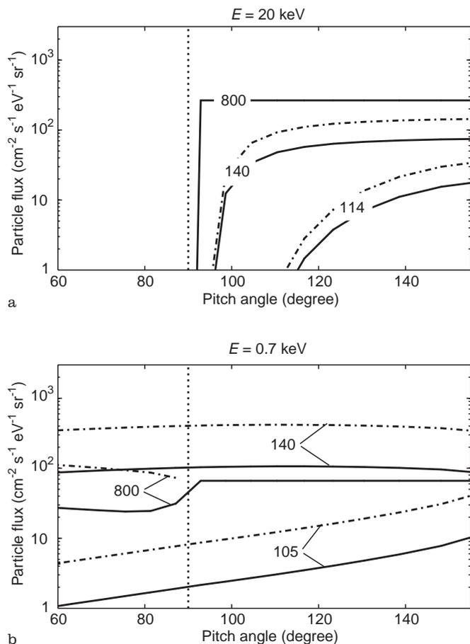
**Fig. 6.** **a** Particle fluxes as a function of pitch angle, for different altitude levels (in Km) and for an energy of 20 keV. Proton flux is shown with *solid lines* and H atom flux is plotted with *dashed-dotted lines*. **b** *idem*, but for an energy of 0.7 keV. The upward fluxes – related to pitch angles lower than 90° – result from collisions
