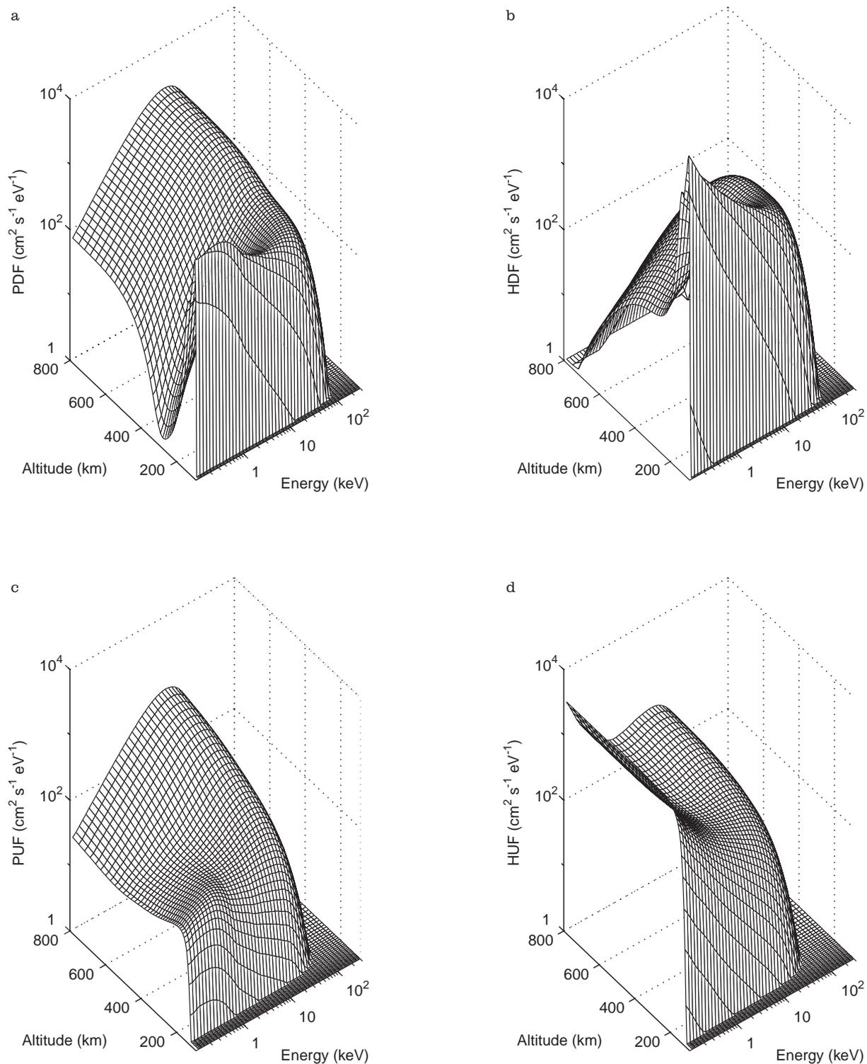
**Fig. 2.** **a** Downward proton flux (PDF), **b** downward H atom flux (HDF), **c** upward proton flux (PUF), and **d** upward H atom flux (HUF), as a function of altitude and energy. These fluxes have been
