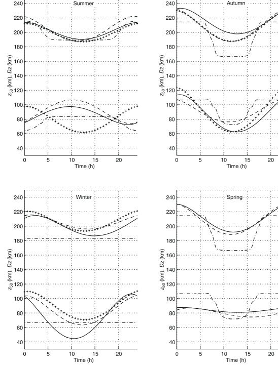
Fig. 5. The results of fitting for various seasons and high (dashed line) and low (continuous line) solar activity are shown. The crossed line corresponds to Lathuillère and Pibaret's model (there is no model for
