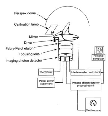
Fig. 1. Schematic diagram of the FPI instrument
