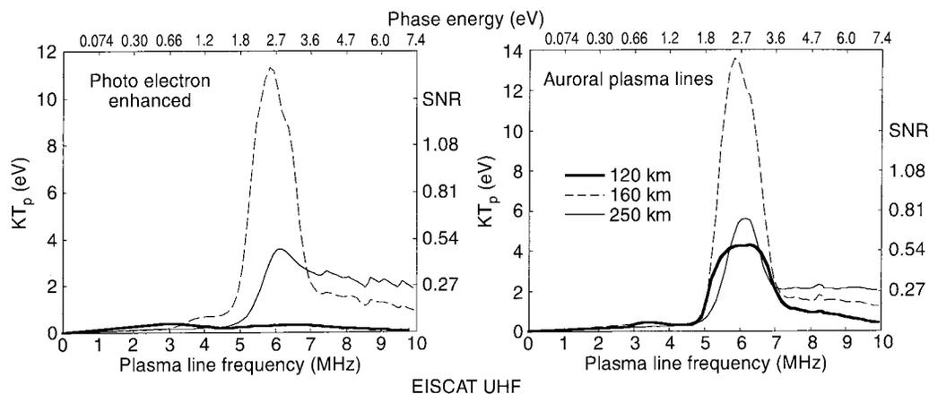
**Fig. 3.** Predicted plasma line strength for the EISCAT UHF radar for daytime and auroral conditions and three different altitudes. The *left y-axis* gives the plasma line temperature in eV, the *right y-axis* the F-region (250 km) signal-to-noise ratio for typical conditions (see
