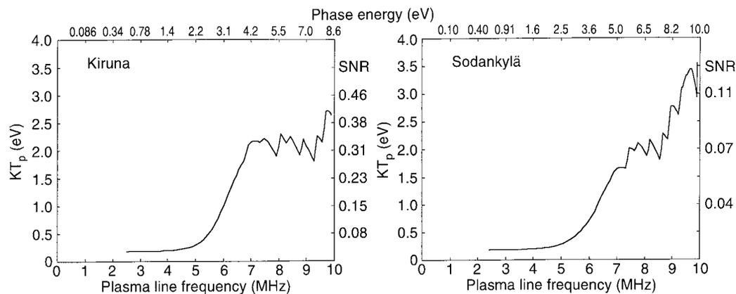
**Fig. 6.** Predicted plasma line strength for the EISCAT UHF remote sites (Kiruna and Sodankylä) for daytime and 250 km altitude. The *left y-axis* gives the plasma line temperature in eV, the *right y-axis* the signal-to-noise ratio for a typical experimental configuration (see
