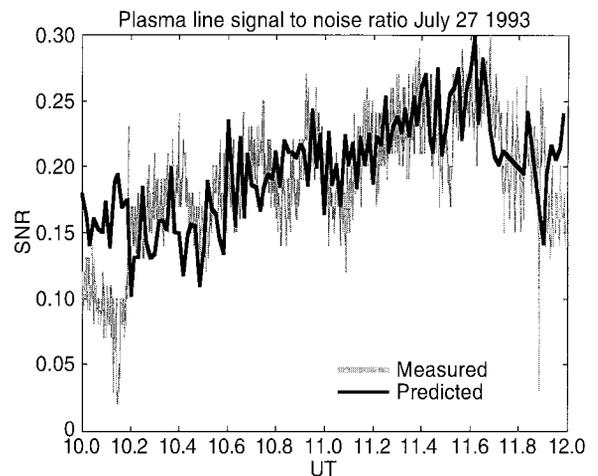
**Fig. 5.** Comparison between measured and predicted signal-to-noise ratio for plasma line measurements at the peak of the F region on 27 July 1993. The *thick gray line* denotes measured SNR, the *thin black line* is the theoretical value calculated from ion line parameters
