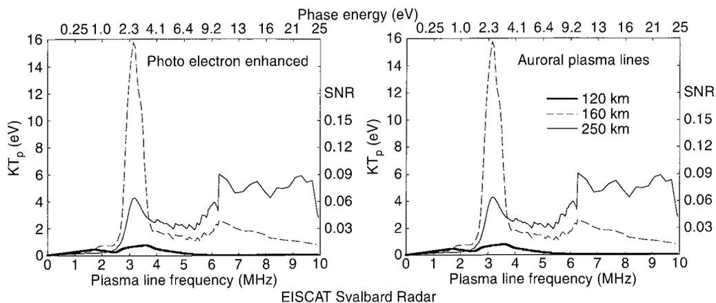
**Fig. 8.** Predicted plasma line strength for the EISCAT Svalbard radar for daytime and auroral conditions and three different altitudes. The *left y-axis* gives the plasma line temperature in eV, the *right y-axis* the F-region (250 km) signal-to-noise ratio for typical
