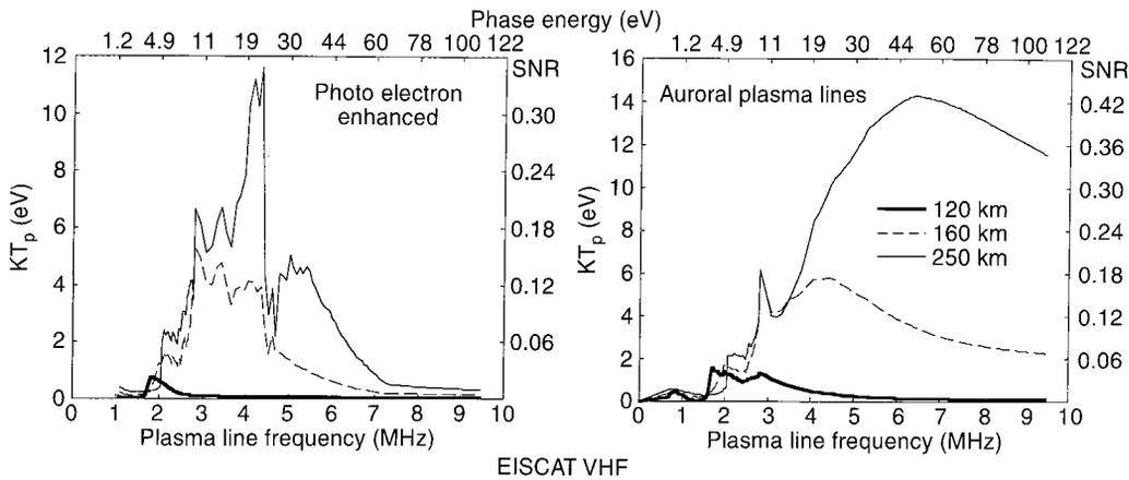
**Fig. 7.** Predicted plasma line strength for the EISCAT VHF radar for daytime and auroral conditions and three different altitudes. The *left y-axis* gives the plasma line temperature in eV, the *right y-axis* the F-region (250 km) signal-to-noise ratio for typical conditions (see
