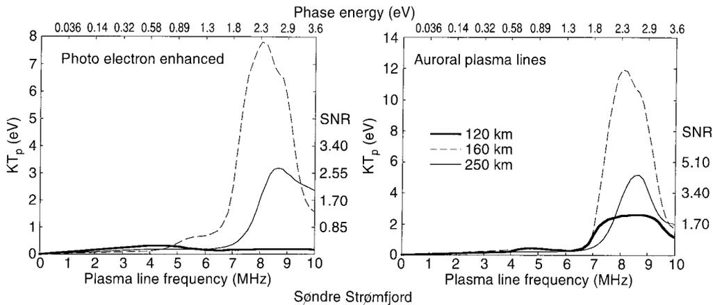
**Fig. 4.** Predicted plasma line strength for the Søndre Strømfjord radar for daytime and auroral conditions and three different altitudes. The *left y-axis* gives the plasma line temperature in eV, the *right y-axis* the F-region (250 km) signal-to-noise ratio for typical
