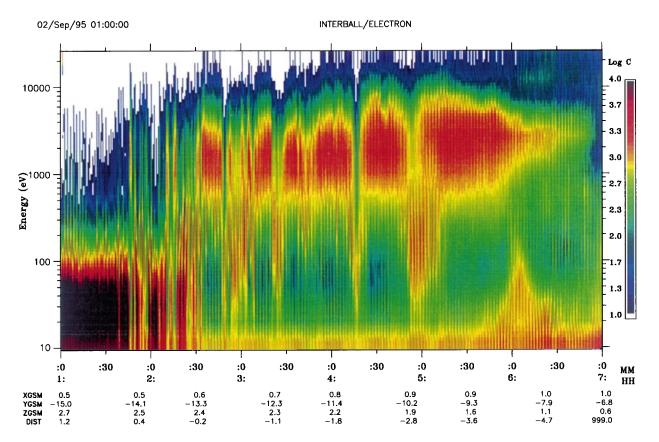
**Fig. 3.** Energy-time spectrogram of electrons in the energy range 10–26000 eV on 2 September 1995 between 01:00:00 and 07:00:00 UT. The data are delivered from the anode of the detector spinning in a plane perpendicular to the ecliptic. Inside the magnetosphere, the
