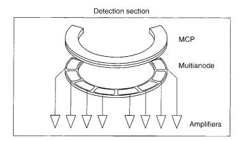
**Fig. 2.** Schematic view of the MCPs located at the output of the analyser and of the sectored anode which allows the discrimination of eight directions covering 180°
