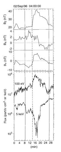
**Fig. 9.** From top to bottom, the magnetic-field components, the total *B* field and the 100 and 5000-eV electron fluxes for 2 September 1995 from 04:00:00 and 04:30:00 UT. The LLBL corresponds to high fluxes of low-energy electron and strong decrease in the keV electron fluxes. Note the strong increase in the *B* field in the LLBL cloud and the bipolar variation of the  $B_x$  component of the magnetic field between 04:14:00 and 0426:40 UT (see text)
