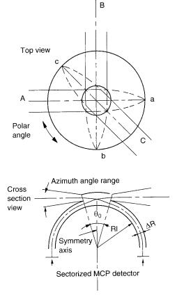
Fig. 1. Schematic views of the top-hat analyser and examples of parallel beam trajectories
