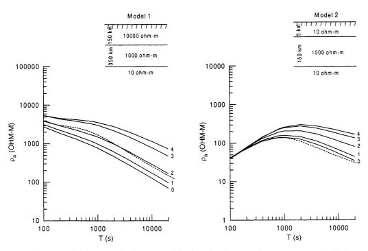
**Fig. 9.** Apparent resistivity curves for the same models of Earth as in Fig. 8. For each model, the *continuous curves* correspond to a gaussian distribution of ionospheric currents, and are denoted in the text as gaussian curves. They are computed at five observation points, and labelled from  $\theta$  to  $\theta$  according to the distance of the point to the center of the electrojet, the curve labelled  $\theta$  corresponding to  $\theta$   $\theta$  times
