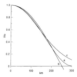
**Fig. 7.** Distribution of E-W ionospheric equivalent currents of the equatorial electrojet: a Quadratic model with a 300 km half-width; b cosine distribution with a 320 km half-period; c gaussian distribution with a 140 km 'standard deviation'
