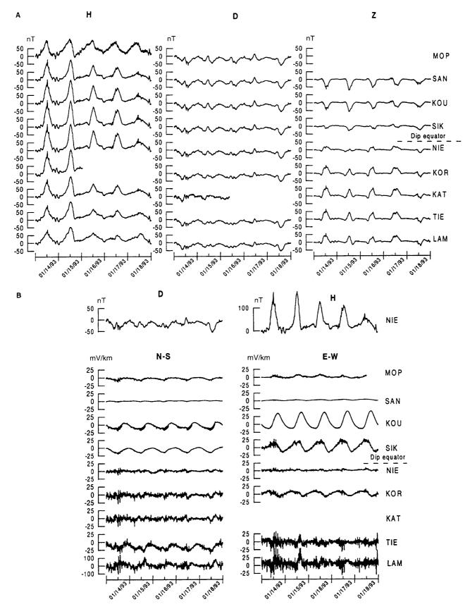
**Fig 3A, B.** Transient variations of the electromagnetic field observed during a 5 day long period of magnetic quietness with a significant magnetic day-to-day variability (January 14, 1993, 00:00 LT to January 18, 1993, 23:59 LT, with a maximum *am* value of 48 nT and
