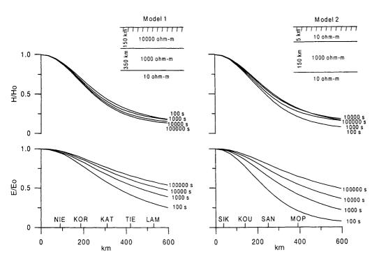
**Fig. 8.** Relative variations of  $E_y$  and  $H_x$  obtained for a gaussian electrojet and for two models corresponding to the mean stratified structure of the Earth below the northern (low resistivity sedimentary
