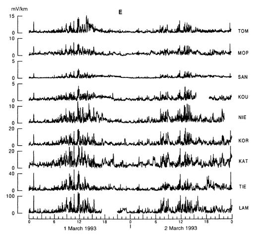
**Fig. 5.** Transient variations of the electric field modulus *E* observed during a disturbed period (March 1, 1993, 00:00 LT to March 2, 1993, 23:59 LT, with a maximum *am* value of 88 nT and an average *am* value of 36 nT)
