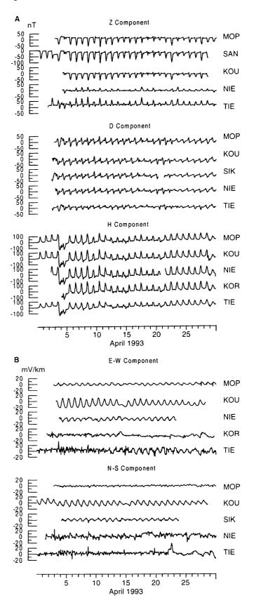
**Fig. 2A, B.** Transient variations of the electromagnetic field observed in April, 1993 at five stations of the electromagnetic profile. **A** Magnetic field; **B** electric field
