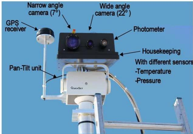
**Fig. 3.** The Pic du Midi camera system.
