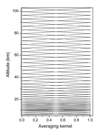
**Fig. 3.** Typical CO averaging kernels for ACE-FTS, using the microwindows shown in Fig. 2, and an Optimal Estimation Method without a priori constraints. The vertical resolution is  $\sim$ 2 km in the troposphere and 4 km above, for a beta angle of  $-50.6^{\circ}$ . At low beta angles, the vertical resolution might reach 6 km at the highest altitudes.
