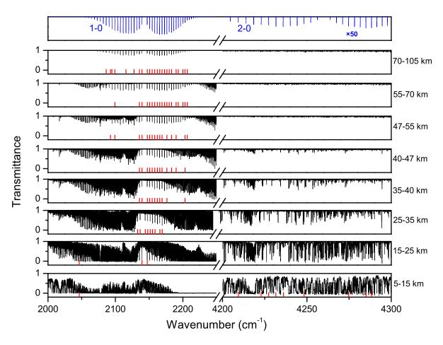
**Fig. 2.** Microwindows (version 2.2., red lines) used to retrieve CO vertical profiles from the ACE-FTS spectra, for a typical occultation sequence spanning from the free troposphere to the mesosphere. The numbers on the right give the approximate altitude range where the microwindows are valid. The top panel shows a simulated CO spectrum (blue), with the absorption in the 2-0 band multiplied by a factor of 50 for clarity.
