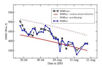
**Fig. 4.** Time series of DSSF<sub>res</sub>, DSSF<sub>meas</sub>, and DSSF<sub>par</sub> for Carpentras at 07:20 UT between 18 July and 19 August 2003. Parameterisation for pure Rayleigh is  $\delta$ =0, W=2.5 g cm<sup>-2</sup>, Uo3=300 DU, parameterisation with aerosols is  $\delta$ =0.09, W=2.5 g cm<sup>-2</sup>, Uo3=300 DU.
