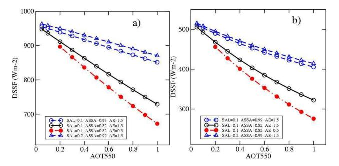
**Fig. 1.** Sensitivity of DSSF to the Aerosol Optical Thickness (AOT) for two values of the Aerosol Single Scattering Albedo (ASSA), two values of the Ånsgröm Exponent (AE) and two values of the Surface Albedo (SAL). Simulations are made with the 6S code for (a)  $SZA=30^{\circ}$  and (b)  $SZA=60^{\circ}$ .
