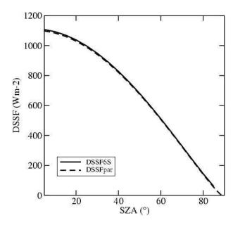
**Fig. 2.** Dependence of DSSF to the Solar Zenith Angle (SZA). 6S simulation and parameterisation for an aerosol-free atmosphere with 300 DU of ozone and 2 g cm<sup>-2</sup> of water vapour.
