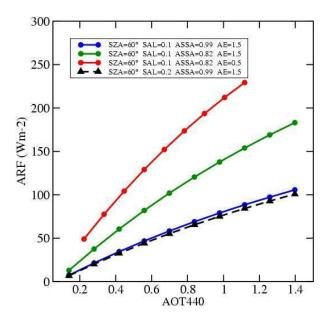
**Fig. 3.** Sensitivity of ARF to AOT440. ARF is computed with the 6S radiative transfer code for several aerosol models, and two values of the Surface Albedo (SAL).
