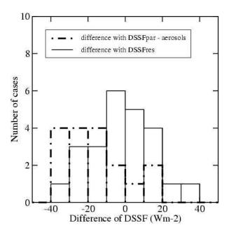
**Fig. 5a.** Histograms of the differences  $DSSF_{par}-DSSF_{meas}$  and  $DSSF_{res}-DSS_{meas}$ , in Carpentras.
