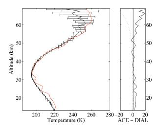
**Fig. 11.** Seasonal average temperature profiles and differences (in K) for the Eureka DIAL (black) and ACE-FTS v2.2 (red) using 16 nights of measurements during the 2004 and 2006 Canadian Arctic ACE Validation campaigns. The error bars are  $1-\sigma$  standard deviations of the mean, also shown as a dotted line in the right-hand panel (in K).
