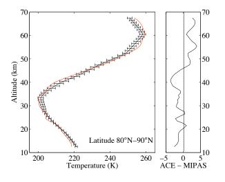
**Fig. 3.** Mean temperature profiles from MIPAS v4.62 (black) and ACE-FTS v2.2 (red) for the latitude region  $80^{\circ}$  N to  $90^{\circ}$  N (left panel) and temperature difference (in K – shown in right panel). Error bars indicate the standard deviation of the mean of the MIPAS temperatures.
