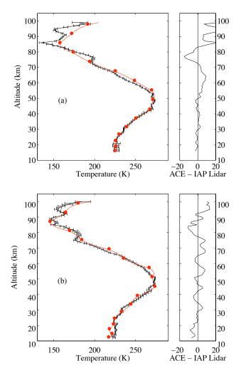
**Fig. 8.** Comparison of temperature profiles from Kühlungsborn lidar (black) and ACE-FTS v2.2 (red) on 21 July 2005 (**a**) and on 24 July 2006 (**b**). The top comparison shows larger differences (in K) in the mesosphere, including an inversion layer measured by the lidar around 78 km.
