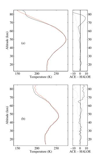
**Fig. 4.** Mean temperature profiles (left panels) for HALOE v19 (black) and ACE-FTS v2.2 (red) and temperature differences (in K, right panels in solid black lines) with standard deviation of the differences (dotted black lines). (a) Results for all 53 coincidences, measurements within 500 km and 4 h. (b) Results from the subset of eight coincidences without the risk of PMC contamination on the HALOE temperature retrievals.
