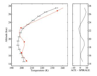
**Fig. 10.** Comparison of ACE-FTS v2.2 (red) temperature profile with SPIRALE balloon-borne (black) temperature measurements (in K) near Kiruna, Sweden on 20 January 2006. Description of plotting convention is given in Fig. 5 caption.
