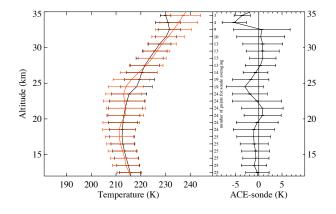
**Fig. 14.** Mean temperature profiles from ACE-FTS v2.2 (red) and radiosondes (black) during the 2005 Canadian Arctic ACE Validation Campaign (left) and the mean of the differences between the two data sets (right). Description of plotting convention is given in Fig. 13.
