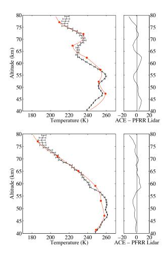
**Fig. 9.** Comparison of temperature profiles (in K) from Poker Flat Research Range (black) and ACE-FTS v2.2 (red) on 28 January 2005 (top) and on 9 September 2005 (bottom). The top comparison shows larger temperature differences than the lower comparison. However, the inversion layer around 70 km is evident in both measurements in the top comparison.
