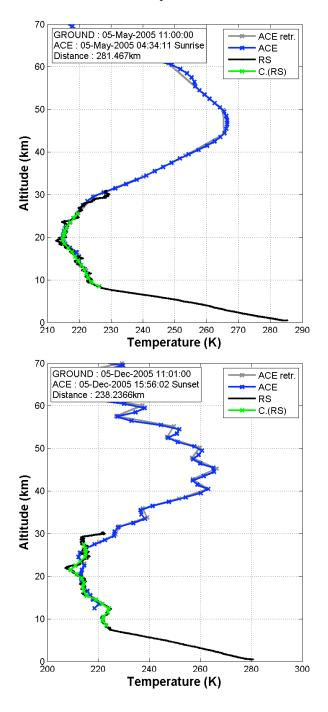
**Fig. 17.** Vertical temperature profile as retrieved from ACE-FTS measurement (grey) and interpolated on 1 km grid (blue) on 5 May 2005 (top panel) and on 5 December 2005 (bottom panel). Collocated temperature profile measured by radiosonde launched from Payerne Alpine station (black) and interpolated to ACE-FTS altitude grid is shown (green).
