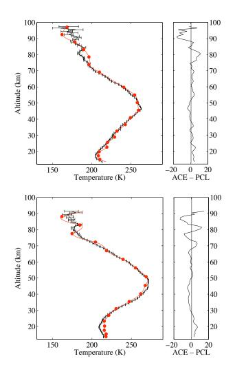
**Fig. 7.** Sample comparisons showing generally good agreement (in K) between the Purple Crow Lidar (black) and ACE-FTS v2.2 (red) temperatures on 1 September 2005 (top). In this case, ACE-FTS misses a small-scale mesospheric inversion. Comparison on 5 May 2006 (bottom), with the unphysical oscillations in the ACE-FTS v2.2 temperatures clearly visible. The agreement between the instruments is particularly good in the mesosphere up to 65 km on this night where no clear inversion is present.
