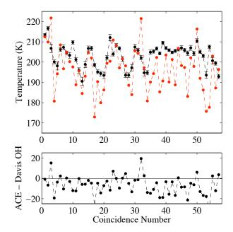
**Fig. 6.** A comparison of 57 coincident Davis OH rotational temperatures (black) with ACE-FTS v2.2 temperatures (red) at 87.5 km altitude (top) and differences (bottom; in K). The error bars on the OH rotational temperature time series are  $1-\sigma$  standard deviation in the nightly mean.
