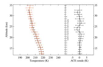
**Fig. 15.** Mean temperature profiles from ACE-FTS v2.2 (red) and radiosondes (black) during the 2006 Canadian Arctic ACE Validation Campaign (left) and the mean of the differences between the two data sets (right). Description of plotting convention is given in Fig. 13.
