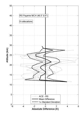
**Fig. 18.** Difference between each pair of ACE-FTS v2.2 and radiosonde temperature profiles at the Alpine station Payerne plotted versus altitude (grey lines). Corresponding mean (plain black line) and  $1-\sigma$  standard deviation (dashed black line) are also shown.
