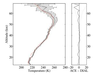
**Fig. 12.** Seasonal average temperature profiles and differences (in K) for the Eureka DIAL (black) and ACE-FTS v2.2 (red) using 5 nights of measurements during the 2005 Canadian Arctic ACE Validation campaign. The error bars are  $1-\sigma$  standard deviations of the mean, also shown as a dotted line in the right-hand panel (in K).
