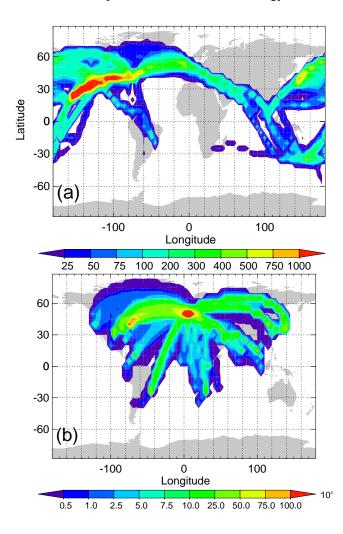
**Fig. 1.** Number of measurements and distribution of flight routes for the **(a)** GASP and **(b)** MOZAIC aircraft programs. Measurements counted over a 5°×5° grid during (a) 1975–1979 and (b) 1994–2001. Note the different colour scales for GASP and MOZAIC flight routes. MOZAIC colour scale needs to be multiplied by 1000 to obtain number of measurements.
