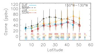
**Fig. 10.** Meridional cross section of mean UT ozone ( $\Delta\theta$ <0 K) (ppbv) for the longitude range 150° W to 130° W as function of season. Vertical bars denote standard deviation. DJF: blue solid line, asterisks, MAM: black dashed line, diamonds, JJA: orange dash-dot line, triangles, SON: red dash-dot-dot line, squares. Averages are only displayed when more than 20 records are available. Number of records is presented at the bottom for each latitude and season, from DJF upward to SON.
