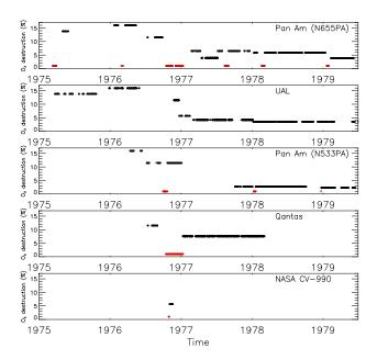
**Fig. 2.** Ozone destruction rates (%) between the probe inlet and the ozone monitor as function of time and aircraft. From top to bottom: Pan Am (N655PA), United Airlines (UAL), Pan Am (N533PA), Qantas, NASA CV-990. Red dots at 1% ozone destruction denote times, when aircraft were flying, but ozone destruction rates were not recorded.
