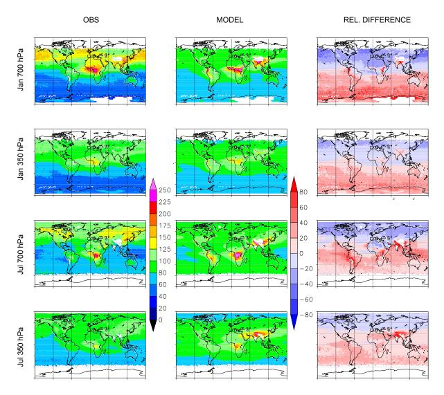
**Fig. 3.** MOCAGE-Climat CO mixing ratios (ppbv) from the T42 simulation versus MOPITT mixing ratios (see text), and relative differences  $(100 \times ((Model - Obs)/Obs))$ , in January (2 upper rows) and July (2 bottom rows), at 700 and 350 hPa. The time versus latitude diagrams are also shown.
