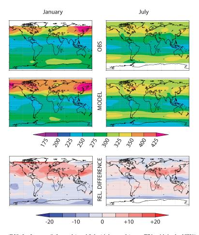
Fig. 14. Total ozone columns (DU) for January (left panels) and July (right panels) on a T21 grid, in the NIWA climatology (top panels, in white no observations), simulated by MOCAGE-Climat (middle panels), and relative differences  $(100 \times (\text{model} - \text{obs})/\text{obs})$ .
