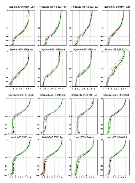
Fig. 17. MOCAGE-Climat vertical profiles of  $O_3$  mixing ratios (ppbv) against Logan (1999a) observations, from 1000 to 10 hPa (black curve,  $\pm 1$  standard deviation as grey curves), at various sites in January (left column), April (middle left), July (middle right), and October (right). MOCAGE-Climat T21 simulations appear as red profiles, T42 simulations as green ones (both axes have a logarithmic scale).
