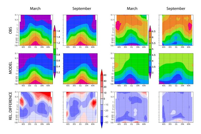
Fig. 2. MOCAGE-Climat T21 zonal monthly mixing ratios against the Grooss and Russel (2005) climatology, and relative differences  $(100 \times ((Model - Obs)/Obs))$ , between 100 and 0.1 hPa, in March (left panels) and September (right panels): first two columns CH<sub>4</sub> (ppmv), and last two columns H<sub>2</sub>O (ppmv).
