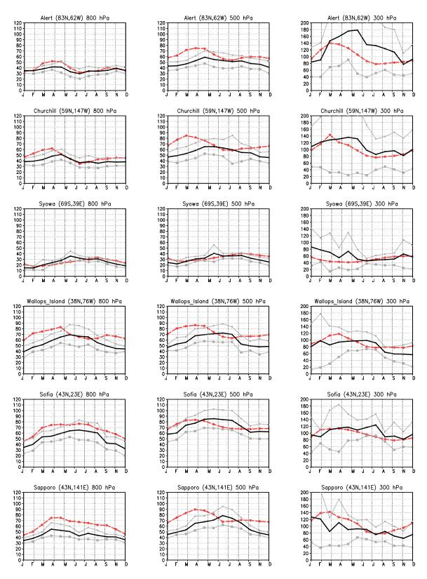
Fig. 19. MOCAGE-Climat monthly  $O_3$  mixing ratios (ppbv) at three different pressure levels, 800 (left), 500 (middle), and 300 hPa (right), against Logan (1999a) observations (black curve,  $\pm 1$  standard deviation as grey curves). MOCAGE-Climat T21 simulations appear as the red curves.
