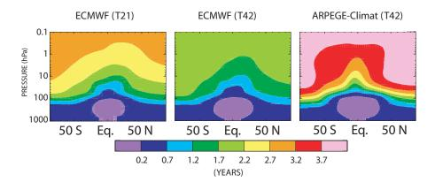
**Fig. 1.** Latitude-pressure cross sections of the resulting age of air (years) when MOCAGE-Climat is driven by the ECMWF operational analyses, at T21 (left) and T42 resolutions (middle), and by outputs from the ARPEGE-Climat GCM at T42 resolution (right). Fields are those of the last year of the simulation.
