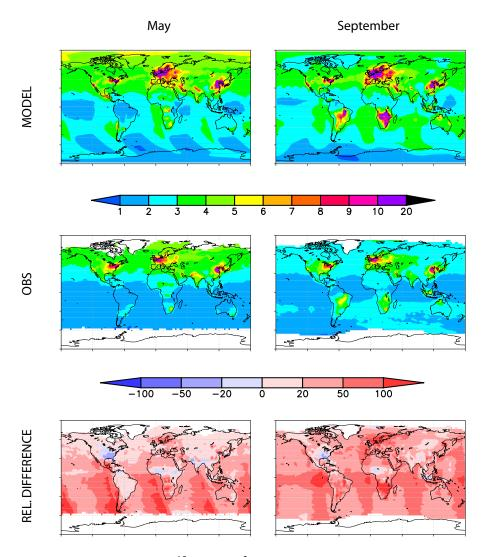
Fig. 9. MOCAGE-Climat T42 total NO<sub>2</sub> columns ( $10^{15}$  molec cm<sup>-2</sup>) versus SCIAMACHY columns at T42 resolution also, and relative differences ( $100 \times ((\text{Model} - \text{Obs})/\text{Obs}))$ , in May (left panels) and September (right panels).
