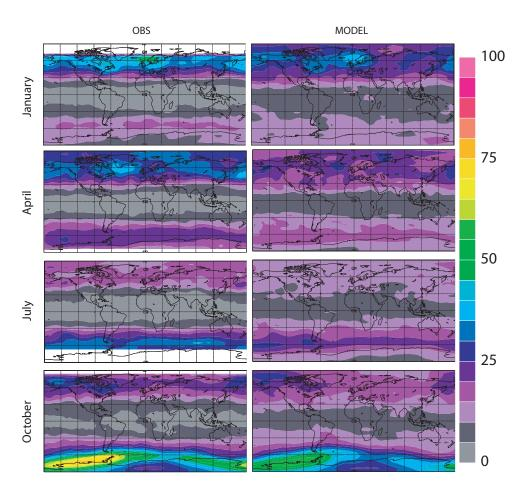
Fig. 15. Standard deviation of the daily total ozone column (DU) for January (first line), April (second line), July (third line), and October (bottom line) on a T21 grid, as observed by TOMS (left panels, in white no observations) and simulated by MOCAGE-Climat (right panels).
