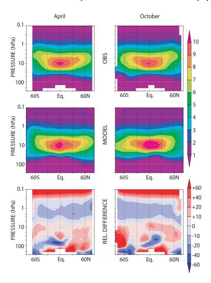
Fig. 16. MOCAGE-Climat T21 zonal monthly mixing ratios of O<sub>3</sub> (ppmv) against the Grooss and Russel (2005) climatology, and relative differences (100×((Model-Obs)/Obs)), between 300 and 0.1 hPa, in April (left panels) and October (right panels).
