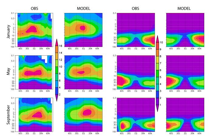
**Fig. 8.** First two columns: MOCAGE-Climat T21 zonal monthly mixing ratios of  $NO_x$  (ppbv) against the Grooss and Russel (2005) climatology, between 100 and 0.1 hPa, in January (upper panels), May (middle panels), and September (lower panels). Last two columns: MOCAGE-Climat T21 zonal monthly mixing ratios of HNO<sub>3</sub> (ppbv) against the Randel et al. (1998) climatology, between 100 and 0.3 hPa, in January (upper panels), May (middle panels), and September (lower panels).
