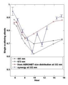
**Fig. 11.** Daytime evolution of single-scattering albedo on 18 May retrieved from the synergy between lidar and sun photometer at 355 nm (left) and 532 nm (right) and from AERONET data (channels 441 nm and 673 nm) using Mie calculation based on AERONET size distribution and complex refractive index given in Table 1. Vertical bars are the standard deviation on hourly averaged data.
