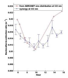
**Fig. 6.** Daytime evolution of BER on 18 May retrieved from the synergy between lidar and sun photometer at 355 nm (left) and 532 nm (right) and from AERONET data (channels 441 nm and 673 nm) using Mie calculation based on AERONET size distribution and complex refractive index given in Table 1. Vertical bars are the standard deviation on hourly averaged data.
