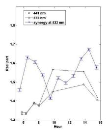
**Fig. 8.** Daytime evolution of the real part of ACRI  $(n_r)$  retrieved from the synergy between lidar, sun photometer and in-situ instruments at 355 nm (left) and 532 nm (right) and from AERONET data (channels 441 nm and 673 nm). Vertical bars are the standard deviation on hourly averaged data.
