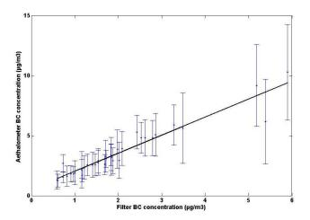
**Fig. 3.** Calibration curve of black carbon concentration measured by aethalometer (BC<sub>a</sub>) against the black carbon concentration measured on filters (BC<sub>f</sub>). Vertical bars indicate standard deviations on aethalometer measurements. The correlation ratio of this fitting is close to 0.96 for a linear law given by BC<sub>a</sub>=1.5 BC<sub>f</sub> + 0.54.
