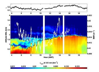
**Fig. 1.** Temporal evolution of the vertical profile of aerosol extinction coefficient at 532 nm above Paris on 18 May 2005 between 03:00 and 20:00 UTC. The upper part of the figure represents the corresponding total aerosol optical thickness. Both the PBL and the residual layer heights are given in a black curve. Daytime evolution of the BER at 532 nm is given in white.
