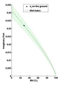
Fig. 13. Evolution of both the real and the imaginary part of ACRI at 532 nm as functions of the relative humidity (RH) based on observation performed between 12:00 and 13:00 UTC on 18 May. The dashed line represents the Hänel parametrisation curve and the filled circle shows the value retrieved on the surface level. The shaded area corresponds to the uncertainties linked to the error on ground computation and on RH.
