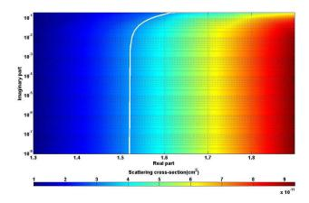
**Fig. 7.** Aerosol scattering cross-sections calculated for various real and imaginary parts of the complex refractive index (colour bar associated to the look-up table) at the wavelength of 532 nm. The mean value of the scattering cross section retrieved from in situ measurements  $(3.37\ 10^{-11}\ cm^2)$  is also given in white for 18 May between 12:00 and 13:00 UTC.
