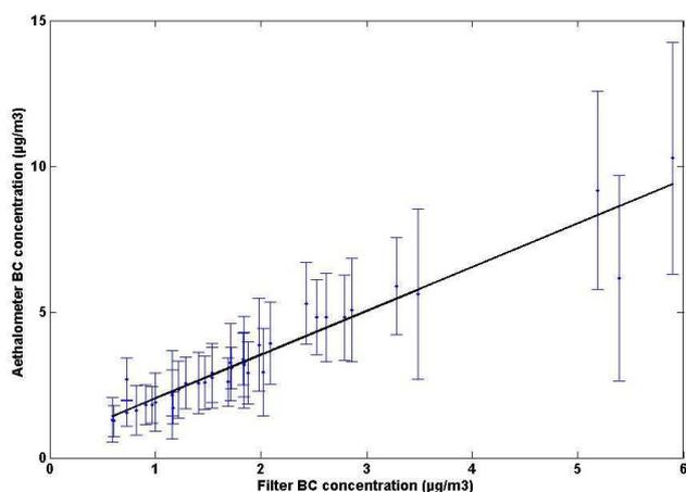
**Fig. 3.** Calibration curve of black carbon concentration measured by aethalometer ( $BC_a$ ) against the black carbon concentration measured on filters ( $BC_f$ ). Vertical bars indicate standard deviations on aethalometer measurements. The correlation ratio of this fitting is close to 0.96 for a linear law given by  $BC_a = 1.5 BC_f + 0.54$ .
