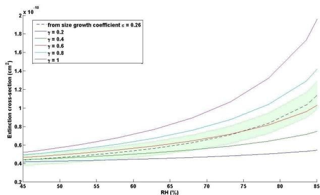
**Fig. 14.** Aerosol extinction cross section against the relative humidity (RH) based on observation performed between 12:00 and 13:00 UTC on 18 May. Colored solid lines represent the Hänel parametrisation curves with different scattering growth coefficients  $\gamma_e$ , whereas the dashed line shows the evolution of the cross section as calculated with Mie model and a size growth coefficient of 0.26. The shaded area corresponds to the uncertainties.
