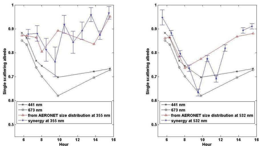
**Fig. 11.** Daytime evolution of single-scattering albedo on 18 May retrieved from the synergy between lidar and sun photometer at 355 nm (left) and 532 nm (right) and from AERONET data (channels 441 nm and 673 nm) using Mie calculation based on AERONET size distribution and complex refractive index given in Table 1. Vertical bars are the standard deviation on hourly averaged data.
