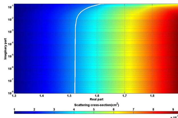
**Fig. 7.** Aerosol scattering cross-sections calculated for various real and imaginary parts of the complex refractive index (colour bar associated to the look-up table) at the wavelength of 532 nm. The mean value of the scattering cross section retrieved from in situ measurements ( $3.37 \cdot 10^{-11} \text{ cm}^2$ ) is also given in white for 18 May between 12:00 and 13:00 UTC.
