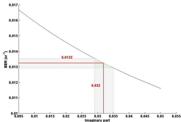
**Fig. 9.** Imaginary part of the complex refractive index at 532 nm retrieved from a mean value of BER between 12:00 and 13:00 UTC on 18 May. The gray band wrapping the curve represents the uncertainty on the retrieved value.
