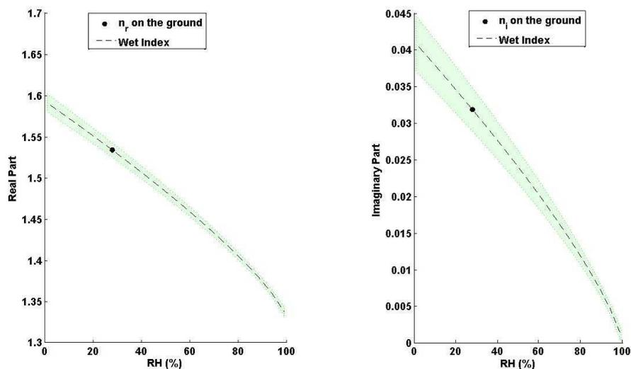
**Fig. 13.** Evolution of both the real and the imaginary part of ACRI at 532 nm as functions of the relative humidity (RH) based on observation performed between 12:00 and 13:00 UTC on 18 May. The dashed line represents the Hänel parametrization curve and the filled circle shows the value retrieved on the surface level. The shaded area corresponds to the uncertainties linked to the error on ground computation and on RH.
