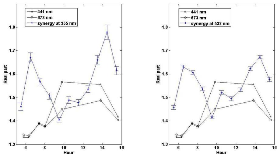
**Fig. 8.** Daytime evolution of the real part of ACRI ( $n_r$ ) retrieved from the synergy between lidar, sun photometer and in-situ instruments at 355 nm (left) and 532 nm (right) and from AERONET data (channels 441 nm and 673 nm). Vertical bars are the standard deviation on hourly averaged data.
