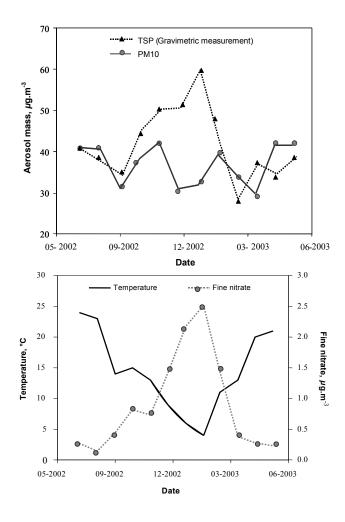
**Fig. 1.** Monthly averages at Florence (July 2002–June 2003). (a) PM-10 obtained with TEOM and TPM by filter gravimetric measurements. (b) TPM nitrate concentrations as a function of ambient temperature.
