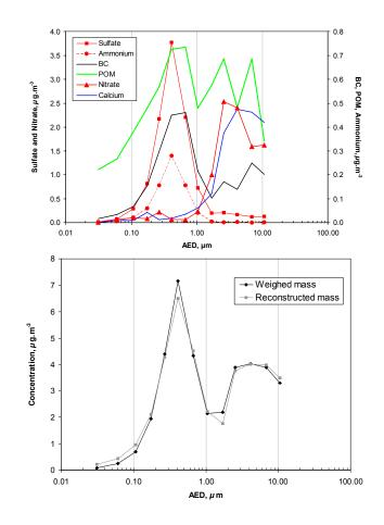
**Fig. 4.** Size distribution in Marseilles (2 July 2005). (a) Mass size distribution of BC, POM, sulphate, nitrate, ammonium, calcium. The association between  $Ca^{2+}$  and  $NO_3^-$  is particularly clear in the coarse mode. (b) Consistency between the actual weighed mass and the reconstructed mass over the whole distribution.
