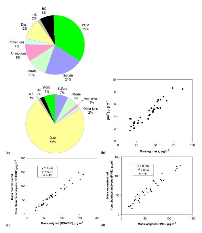
**Fig. 3.** Mass closure for Pek3 experiment (August 2004), all samples. (a) Mean chemical composition of the coarse (down) and fine (up) modes. (b) Missing mass/Ca<sup>2+</sup> correlation in the coarse mode. (c) Mass closure of the coarse mode: Consistency between the actual weighed mass and the reconstructed mass. (d) Mass closure of the fine mode after k adjustment (k=1.65).
