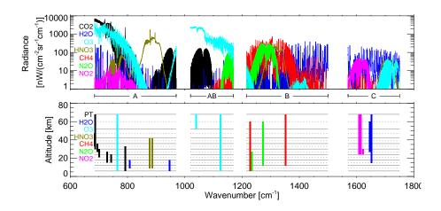
**Fig. 1.** The upper plot shows the major absorbing molecules in the MIPAS spectra for 21 km tangent altitude and the lower plot shows the spectral locations and tangent altitude range of the microwindows used for the MIPAS retrievals (note that the actual spectral width of each microwindow – maximum  $3 \text{ cm}^{-1}$  – is too narrow to be shown to scale on these plots). A, AB, B and C are the first 4 MIPAS bands.
