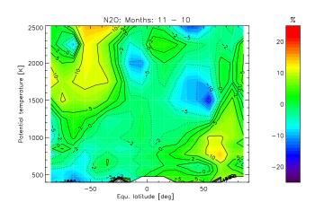
Fig. 9. Day–Night differences in retrieved  $N_2O$  on equivalent latitudes versus potential temperature. Differences represent mean values over the whole observational period (July 2002–March 2003).
