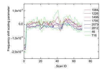
**Fig. 6.** Fit of the frequency scaling factor as a function of the scan identification number (ID) for different sets of spectral points (depending on the analysed species and on the measurement band). Different colours are used for the fits that use few points (green curves), medium number of points (red curves) and large number of points (blue curves).
