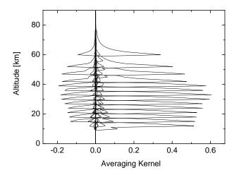
**Fig. 10.** Averaging kernels for the ozone retrieval in the case of  $20^{\circ}$  N–65° N latitude band in July.
