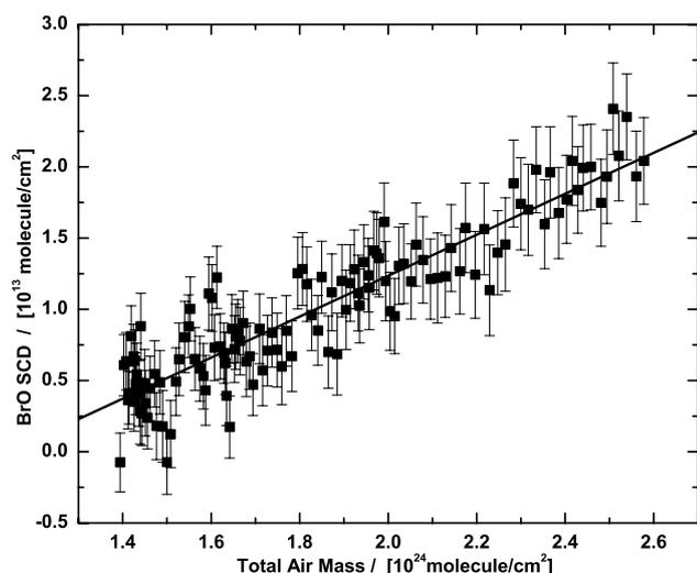
**Fig. 8.** Measured BrO absorption as a function of the calculated total air mass observed for a SZA range between  $84.27^\circ$  and  $87.52^\circ$  at balloon float altitude (33.5 km) over Aire sur l'Adour on 9 October 2003. The slope of the least-square-fitted data results in the average BrO mixing ratio of  $(14.4 \pm 0.7)$  pptv above float altitude.
