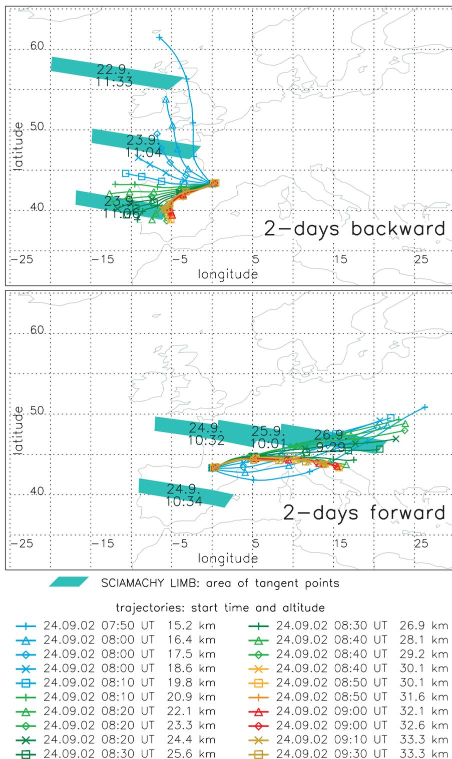
**Fig. 1.** Two days backward (upper panel) and forward (lower panel) air mass trajectories for TRIPLE ascent observations at Aire sur l'Adour, France, on 24 September 2002. Envisat/SCIAMACHY orbit numbers matching with the TRIPLE trajectory are 2940, 2954, 2968, 2982, 2995, and 2996. The light blue rectangles represent the area probed by SCIAMACHY limb observations.
