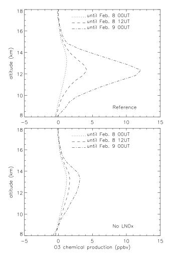
**Fig. 5.** Vertical profile of the mean accumulated chemical ozone production in Grid 2 of the RAMS model until 8 February 00:00 UT, 8 February 12:00 UT, 9 February 00:00 UT. (a) "reference" run. (b) "no  $LNO_X$ ". run.
