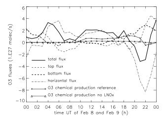
**Fig. 8.**  $O_3$  instantaneous fluxes on each side of the domain shown in Fig. 7 between 8 February 00:00 UT and 9 February 00:00 UT for the "reference" run. The positive sign of the flux means that the flux is entering the domain. Also shown are the instantaneous  $O_3$  chemical production within the domain for both simulations and the total of each flux including the  $O_3$  production (solid line) for the "reference" run.
