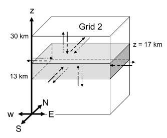
**Fig. 7.** Schematic of the box used to calculate the ozone budget in the TTL (shaded domain delimited at the bottom by the 13 km level, at the top by the 17 km level and on the sides by the boundary of Grid 2. The net contribution (inflowing flux or outflowing flux) on the budget for each side of the domain is indicated by the sense of the corresponding bold arrows.
