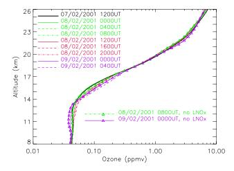
**Fig. 1.** Temporal evolution of the  $O_3$  mean profile in the vertical range (8 km; 26 km) computed at regular 4 h time intervals by RAMS in Grid 2 between 8 February 2001 at 00:00 UT and 9 February 2001 at 04:00 UT. The initial state is also shown (black line). The horizontal scale is logarithmic.
