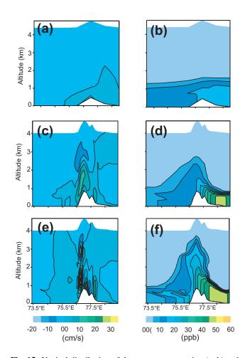
**Fig. 15.** Vertical distribution of the tracer concentration (ppb) and vertical velocity (cm s<sup>-1</sup>) at  $10^{\circ}$  N latitude and between  $73^{\circ}$  E and  $78.5^{\circ}$  E, respectively, obtained with the 1-grid simulation (run A) referred to as S1 (a) and (b), with the 2-grid reference simulation (run B), referred to as S2 (c) and (d) and with the high resolution simulation (run C), referred to as S3 (e) and (f) at 12:00 UTC on 7 March 1999.
