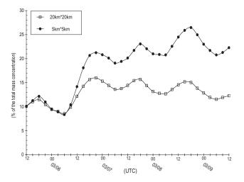
**Fig. 16.** Diurnal evolution of the mean mass concentrations (normalized by the total mass concentration) of the Madras tracer above 1 km a.s.l. as a function of time for run B (open squares) and run C (filled circles).
