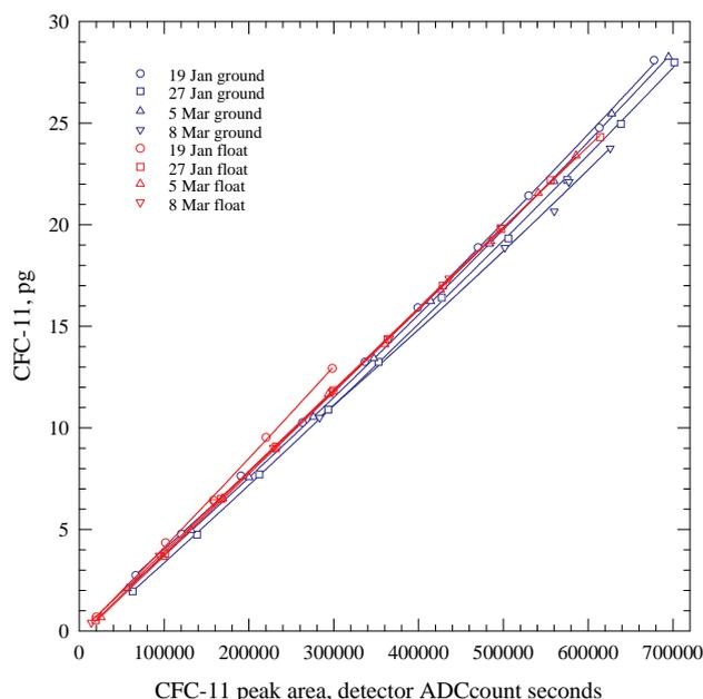
**Fig. 1.** DIRAC in-flight CFC11 response curves for 19 January, 27 January, 5 March and 8 March used to calibrate the in situ CFC11 measurements. The x-axis is peak area expressed in units of detector ADCcount seconds, the y-axis is mass of CFC-11 measured in the calibration gas, expressed in pg of CFC-11.
