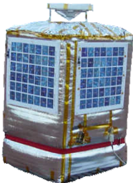
Fig. 1. SAOZ long duration balloon payload. The cone at the top of the instrument defines a 360^\circ azimuth, -10^\circ , +10^\circ elevation FOV within which the full sun could be observed at sunrise and sunset without additional tracking system.
