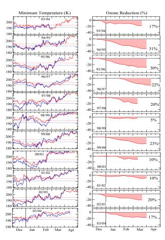
**Fig. 4.** Left: minimum ECMWF temperature at 475 K (red) and 550 K (blue) north of 30° N and limits for NAT PSC formation. Right: Total ozone reduction in the vortex since 1993/1994 from the measurements of the SAOZ stations by comparison to REPROBUS (shaded pink).
