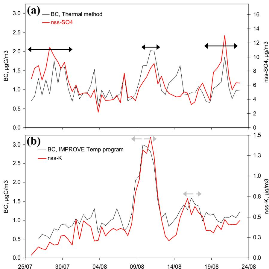
**Fig. 2.** BC from thermal method and nss-SO<sub>4</sub> concentrations (a); BC from thermo-optical IMPROVE method and nss-K (b) at the MBL site for the duration of the MINOS campaign. Black arrows correspond to the anthropogenic influence. Grey arrows correspond to the 2 biomass burning events of the campaign.
