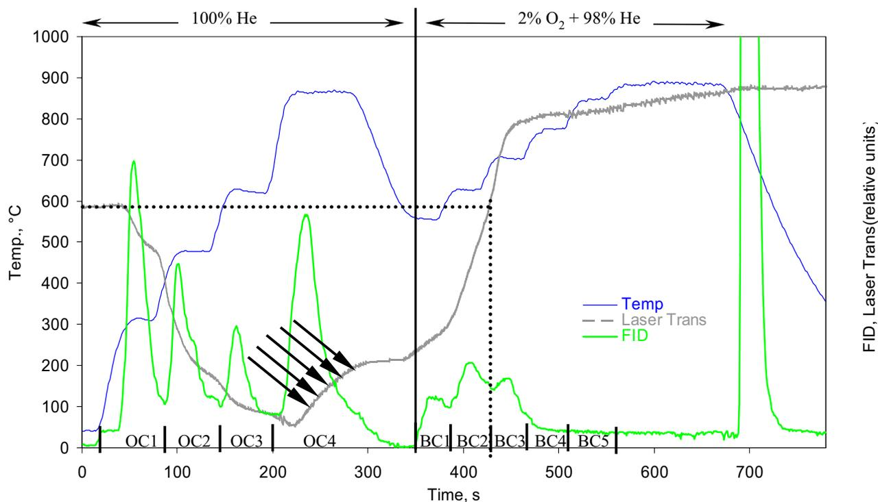
**Fig. 1.** NIOSH temperature program on a quartz filter sampled during MINOS. Black arrows indicate increase in laser transmission (BC loss) at the last temperature step (870°C) under pure helium. OC1-5 and BC1-5 described in Table 1 have been reported here for each temperature step. The optical correction performed by the instrument is reported here (black dotted line) and represent the initial transmittance of the filter.
