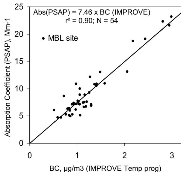
**Fig. 3.** Correlation between BC concentration (IMPROVE Temp prog.) and absorption measurements performed in the field from PSAP. PSAP data are corrected from multiple scattering following the recommendation of Bond et al. (1999).
