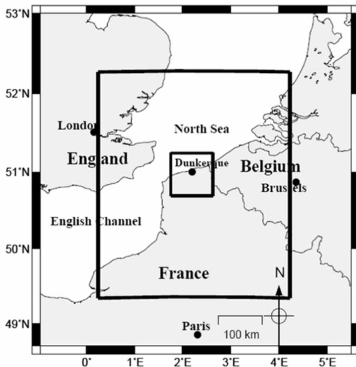
**Fig. 1.** Geographical position of the studied area. The two Meso-NH-C nested models used for the numerical simulation are represented by the two black contours. The 5-km lower horizontal resolution model covers the South-East of England, North of France and part of Belgium. The 1-km higher horizontal resolution model covers the Dunkerque area.
