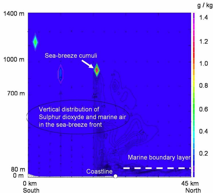
**Fig. 10.** 45 km of vertical south-north cross section computed by the model, at 12:00 UTC and from 0 to 1400 m, of the condensed water in g/kg (colours), with the SO<sub>2</sub> concentration in ppbv (isolines) and the projection of the wind speeds in the cross section (vectors). The sea-breeze front can be visualized by the vertical distribution of SO<sub>2</sub> and at its top can be seen a sea-breeze cumuli.
