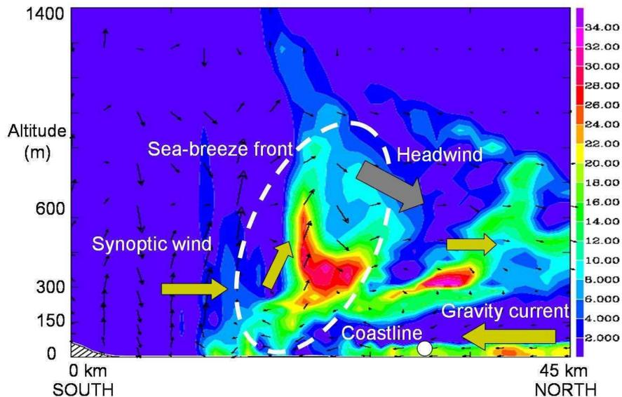
**Fig. 7.** North-south vertical cross section of industrial SO<sub>2</sub> concentrations in ppbv (colour scale) simulated by the model, with the wind velocity in the cross section (vectors) at 14:00 UTC. The south-north distance along the abscissa axis is 45 km. The coastline is represented by the white dot.
