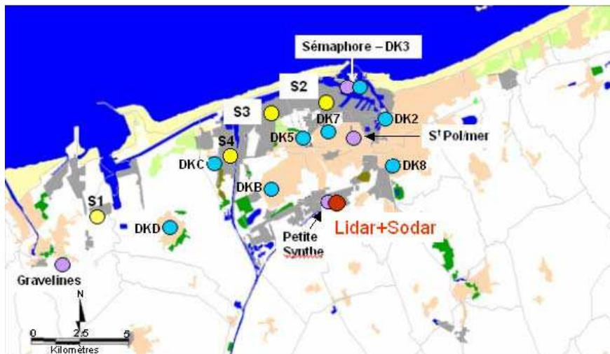
**Fig. 2.** Position of the lidar and sodar instruments (red dot) and location of the ATMO Nord – Pas-de-Calais and Météo-France ground stations in the Dunkerque area: the meteorological stations are represented by violet dots and the stations measuring the pollutant concentrations by blue dots. The yellow dots highlight the major sources of emitted SO<sub>2</sub>.
