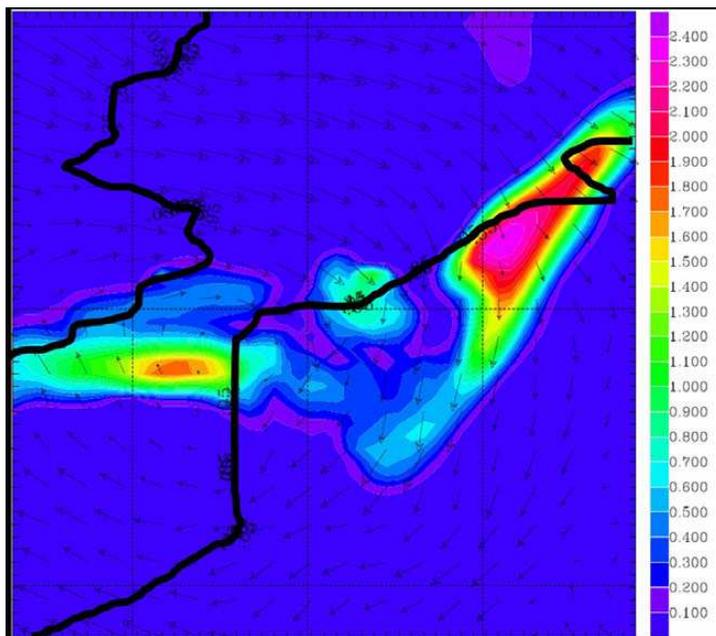
**Fig. 9.** Horizontal cross section of the SO<sub>2</sub> concentration in ppbv (colour scale) and the wind velocity (black arrows) at 06:00 UTC on 16 September at 300 m. The black lines represent the coastlines of the English Channel and the North Sea.
