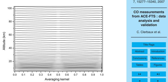
**Fig. 3.** Typical CO averaging kernels for ACE-FTS, using the microwindows shown in Fig. 2, and an Optimal Estimation Method without a priori constraints. The vertical resolution is  $\sim 2 \text{ km}$  in the troposphere and 4 km above, for a beta angle of  $-50.6^{\circ}$ . At low beta angles, the vertical resolution might reach 6 km at the highest altitudes.
