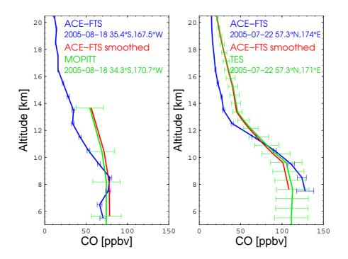
**Fig. 14.** Examples of co-located CO vertical mixing ratio profiles for ACE-FTS (blue) and two nadir-looking instruments (green): MOPITT (left) and TES (right). The retrieval errors are also reported (horizontal blue bars show ACE-FTS fitting errors from v2.2, and horizontal green bars at each retrieved level for the nadir-looking instrument). The red curve represents the convolution of the ACE-FTS profile with the averaging kernel function of the nadir-viewing instrument.
