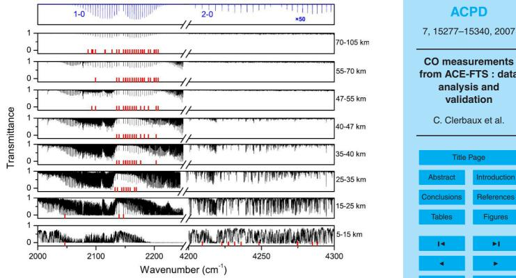
Fig. 2. Microwindows (version 2.2., red lines) used to retrieve CO vertical profiles from the ACE-FTS spectra, for a typical occultation sequence spanning from the free troposphere to the mesosphere. The numbers on the right give the approximate altitude range where the microwindows are valid. The top panel shows a simulated CO spectrum (blue), with the absorption in the 2-0 band multiplied by a factor of 50 for clarity.
