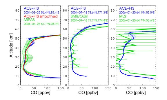
**Fig. 17.** Examples of co-located CO vertical mixing ratio profiles for ACE-FTS (blue) and three limb-looking instruments (MIPAS, SMR and MLS; in green). The retrieval errors are also reported (horizontal blue bars for ACE-FTS fitting errors from v2.2 files, and horizontal green bars for each limb-instrument). As MIPAS data are less vertically resolved, the ACE-FTS profile was smoothed by the MIPAS averaging kernels (in red).
