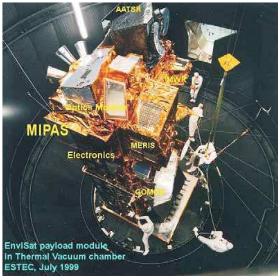
Fig. 1. The MIPAS instrument on top of ENVISAT surrounded by other instruments (AATSR, MWR, MERIS); at the top the optics module with the two baffles is recognized, below the electronics module is fixed on the satellite structure (provided by ESA).
