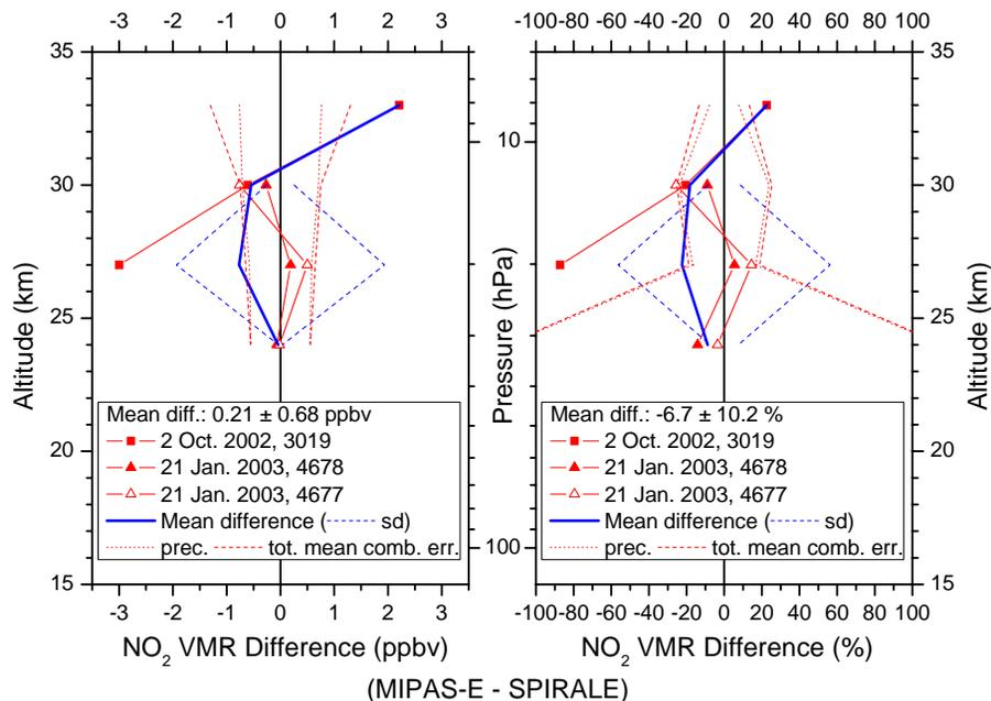
**Fig. 5.** Differences of all comparisons between SPIRALE and MIPAS-E. An ascent profile of SPIRALE from 2 October 2002 is compared to a MIPAS-E limb scan performed during orbit 3019. The SPIRALE profile from 21 January 2003 has been compared to MIPAS-E observations carried out during orbits 4677 and 4678.
