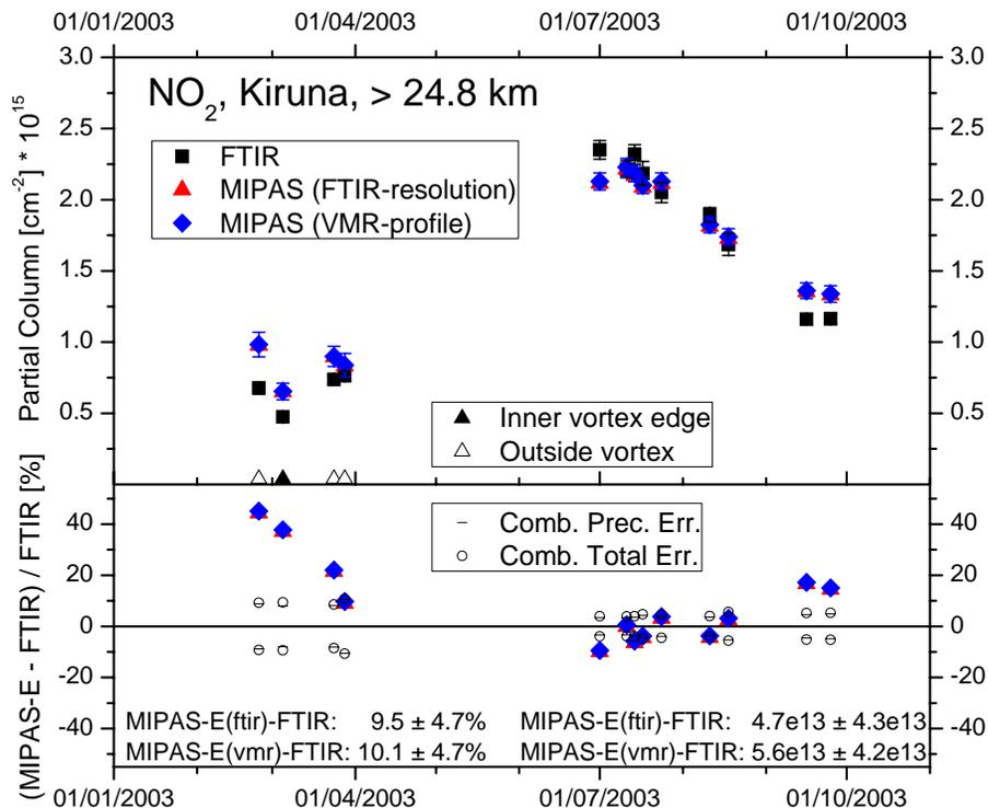
**Fig. 16.** Comparison of NO<sub>2</sub> partial column amounts above 24.8 km to integrated MIPAS columns for the year 2003, measured at Kiruna (68° N, Sweden). MIPAS partial columns have been calculated from both the smoothed profile (MIPAS(FTIR-resolution)) and from the unsmoothed profile (MIPAS(VMR-profile)).
