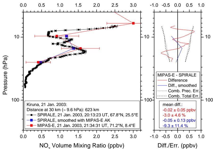
**Fig. 4.** Comparison of NO<sub>2</sub> profiles measured by SPIRALE and MIPAS-E (orbit 4678) on 21 January 2003. The highly resolved vertical profile of SPIRALE has been smoothed with the MIPAS-E averaging kernel matrix.
