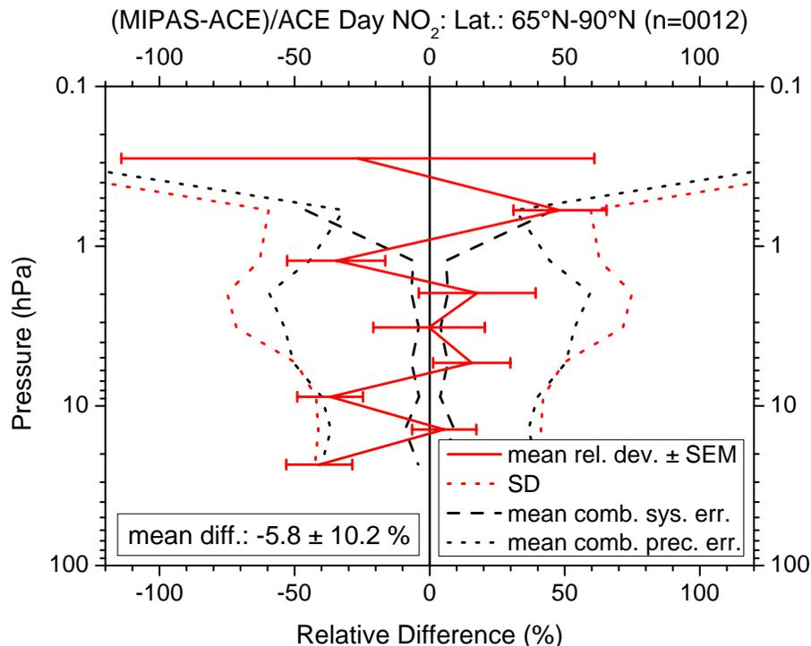
**Fig. 14.** Mean relative difference (including the standard error of the mean, SEM) of MIPAS and ACE NO<sub>2</sub> profiles (12 collocations) between 65° and 90° N latitude in February and March 2004 (red solid line). Random (black dotted line) and systematic (black dashed line) parts of the combined errors are shown together with the standard deviation (red dotted line). Some significant systematic differences appear mainly below about 6 hPa pressure altitude (about 32 km).
