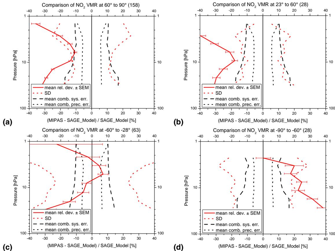
**Fig. 12.** Mean relative differences (including the standard error of the mean, SEM) between MIPAS and SAGE II for different latitude regions in the northern hemisphere (top) and the southern hemisphere (bottom). Standard deviation (SD) and mean combined precision and systematic errors are plotted, too.
