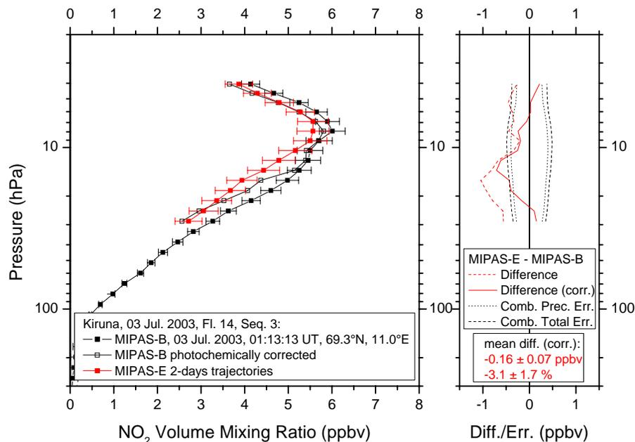
**Fig. 2.** Trajectory comparison for the MIPAS-B flight carried out from Kiruna on 3 July 2003. The MIPAS-B NO<sub>2</sub> values have been transferred to the time and location of the individual MIPAS-E observations with the help of KASIMA model calculations. The mean 2-days trajectory MIPAS-E profile (consisting of several averaged coinciding profiles) can then be compared to the accordingly corrected MIPAS-B profile. The mean difference value is calculated over all coincident altitudes.
