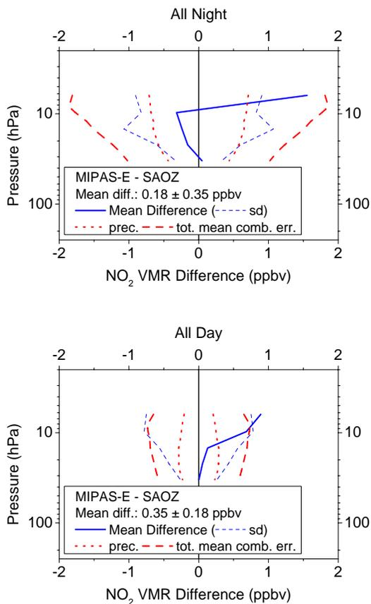
**Fig. 7.** NO<sub>2</sub> measured differences between MIPAS and SAOZ for all MIPAS night (top panel) and MIPAS day (bottom panel) comparisons.
