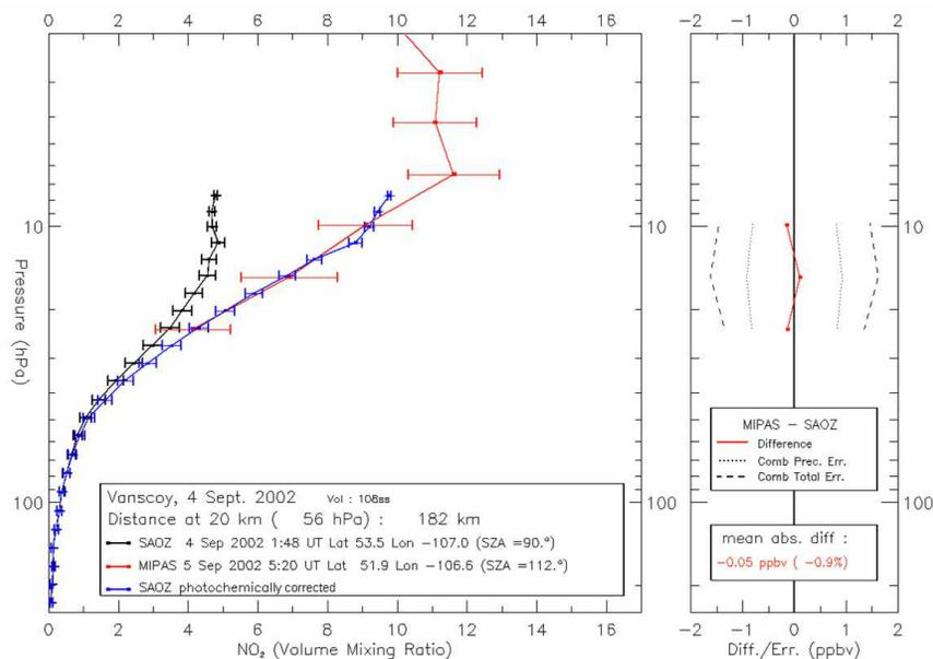
**Fig. 6.** Comparison of SAOZ and MIPAS NO<sub>2</sub> measurements above Vanscoy (Canada, 54° N) on 4 September 2002. The SAOZ sunset observations were photochemically corrected to fit the MIPAS nighttime measurements.
