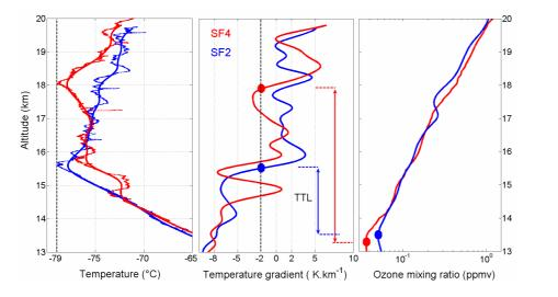
**Fig. 3.** Temperature (micro-SDLA raw and smoothed data), temperature gradients and ozone profiles for both flights, SF2 (in blue) on 13 February and SF4 (in red) on 24 February 2004.
