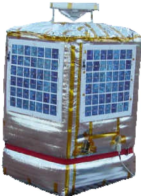
**Fig. 1.** SAOZ long duration balloon version. The cone at the top of the instruments defines a  $360^\circ$  azimuth,  $+10^\circ$ ,  $-10^\circ$  elevation FOV within which the full sun could be observed at sunrise and sunset without additional tracking system.
