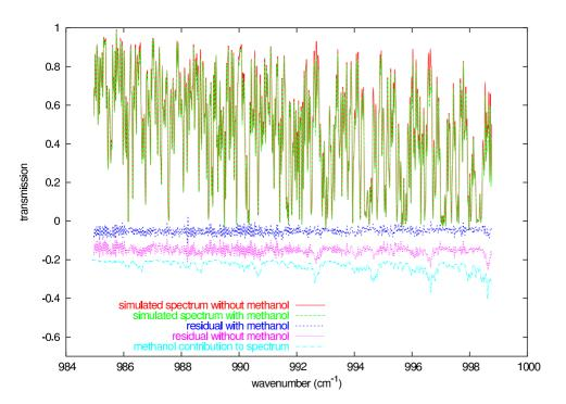
**Fig. 1.** Simulated spectra with methanol included or excluded in the calculation. The corresponding residuals (observed – calculated) and the computed contribution of CH<sub>3</sub>OH to the spectrum using the retrieved vmr are plotted (shifted downwards for clarity).
