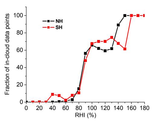
**Fig. 6.** Cloud presence fraction as a function of relative humidity over ice measured by the Polar Nephelometer. If the probe, at a given RHI, observes an extinction coefficient exceeding 0.05 km<sup>-1</sup> during four consecutive seconds the data point is considered a cloudy data point. Only data during straight and level flight segments are included.
