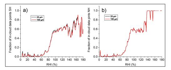
**Fig. 5.** Cloud presence fraction as function of relative humidity over ice for different crystal size thresholds as measured by the PMS-2D probe. If the probe, at a given RHI, observes any crystals having a size equal to or larger than the indicated thresholds found in the figure labels the data point is considered a cloudy data point. Data from SH (a) and from NH (b). Note that in Fig. 5b the black line, representing the  $25 \, \mu m$  threshold, is covered by the red line.
