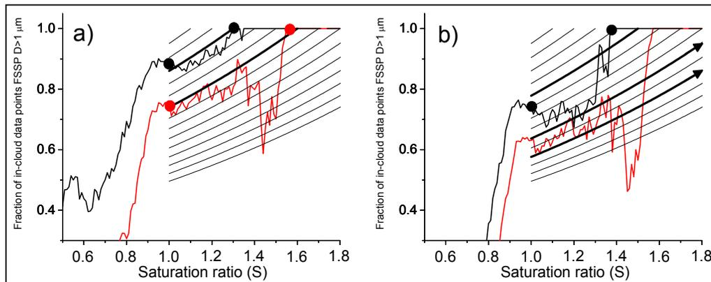
**Fig. 8.** Comparison of the cloud presence fraction observed in the SH and NH campaigns for same FSSP-300 threshold diameters,  $0.5 \mu\text{m}$  (a) and  $1 \mu\text{m}$  (b). The thin lines are calculated distributions of CPF based on Eq. (5) and using  $S_0 = 2$ . Arrows and markers as in Fig. 7.
