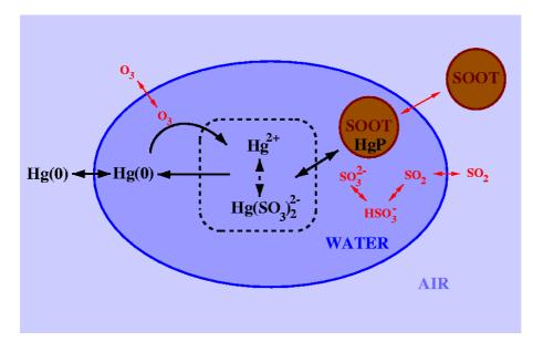
Fig. 1. Schematic of the Petersen et al. (1995) mercury chemistry model.
