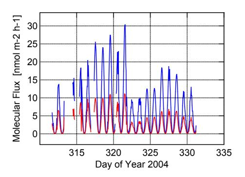
**Fig. 6.** Molecular fluxes of  $NO_2$  (blue line) and HONO (red line) estimated from photolysis of nitrate at Browning Pass during the campaign.
