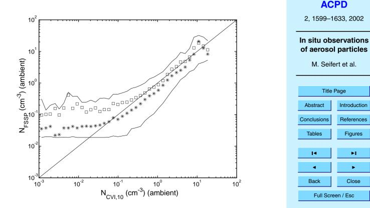
**Fig. 2.** Comparison of the ice particle concentration obtained from the CVI and the FSSP-300. A lower size limit of  $4 \mu m$  was chosen for the FSSP-300 data since it gave the best agreement  $N_{FSSP}$  and  $N_{CVI,10}$ . Averages shown as open squares and medians as stars. The two thin lines correspond to the 10th and 90th percentiles. The dash-dotted line illustrates a 1:1 relation between  $N_{FSSP}$  and  $N_{CVI,10}$ .
