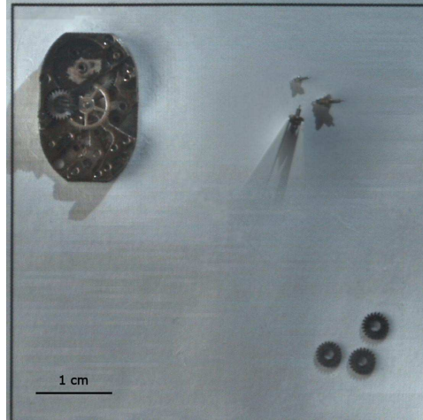
Figure 6. Dynamic mosaic of the benchmark: 1100x1100 pixels, 50\mu\text{m}/\text{pixels} , 55mm x 55mm.
