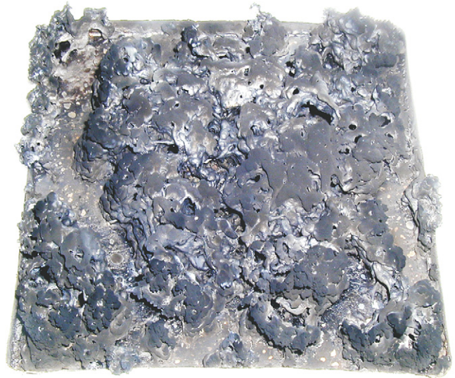
Fig. 7. Photograph of the residue obtained after combustion of the mixture PMMA–9% OP930–6% Al 2 O 3 .
