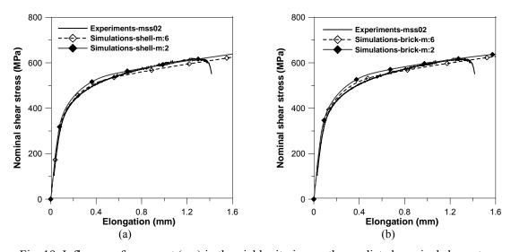
Fig. 19. Influence of exponent (*m*) in the yield criterion on the predicted nominal shear stress-deformation behaviour in (a) shell element model, and (b) brick element model
