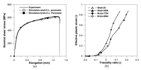
Fig. 15 (a) Experimental and numerical nominal shear stress vs. elongation curves after including failure parameter, and (b) comparison of plastic strain ( $\bar{\varepsilon}$ ) vs. stress triaxiality ( $\sigma_{\scriptscriptstyle m}/\bar{\sigma}$ ) between shell and brick element simulations of shear test
