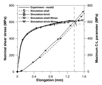
Fig. 13. Correlation of nominal shear stress-elongation curves from experiments and simulations (both shell & brick elements) including plots of  $W_{\rm max}$ , for in-plane shear test
