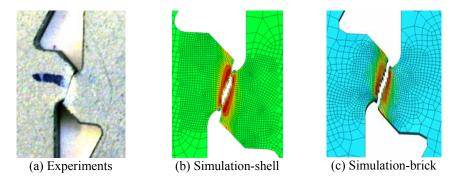
Fig. 18. Comparison of fractured shear zone from experiments, mss02, and simulations
