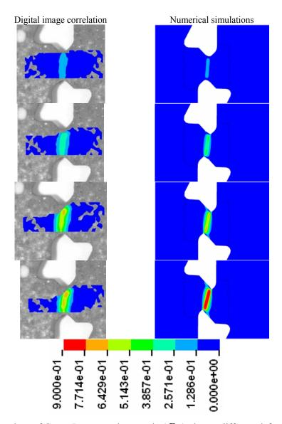
Fig. 16. Comparison of Green-Lagrange shear strain ( $E_{xy}$ ) plots at different deformation stages between digital image correlation (for mss02) and numerical simulations representing with the same colour scale
