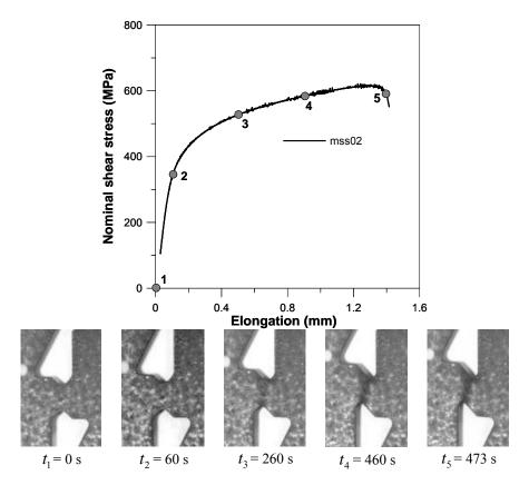
Fig. 10. Sequence of digital images for a quasi-static in-plane shear test, mss02
