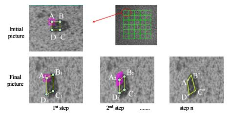
Fig. 5. Field determination principle of DIC
