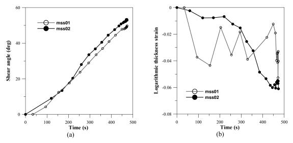
Fig. 11 (a) Shear angle vs. time, and (b) logarithmic thickness strain vs. time, evaluated from the estimated displacement field for the two duplicate shear tests
