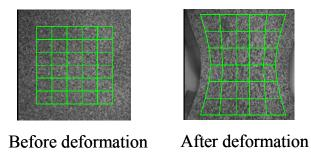
Fig. 4. Schematic representation of FE-based DIC
