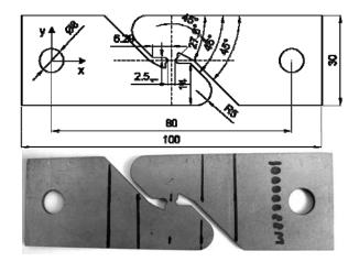
Fig. 2. Geometry of the in-plane shear test specimen
