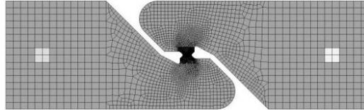
Fig. 14. FE model of the in-plane shear specimen
