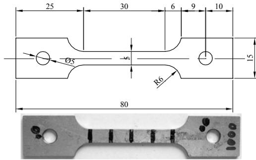
Fig. 1. Geometry of the uniaxial tensile test specimen
