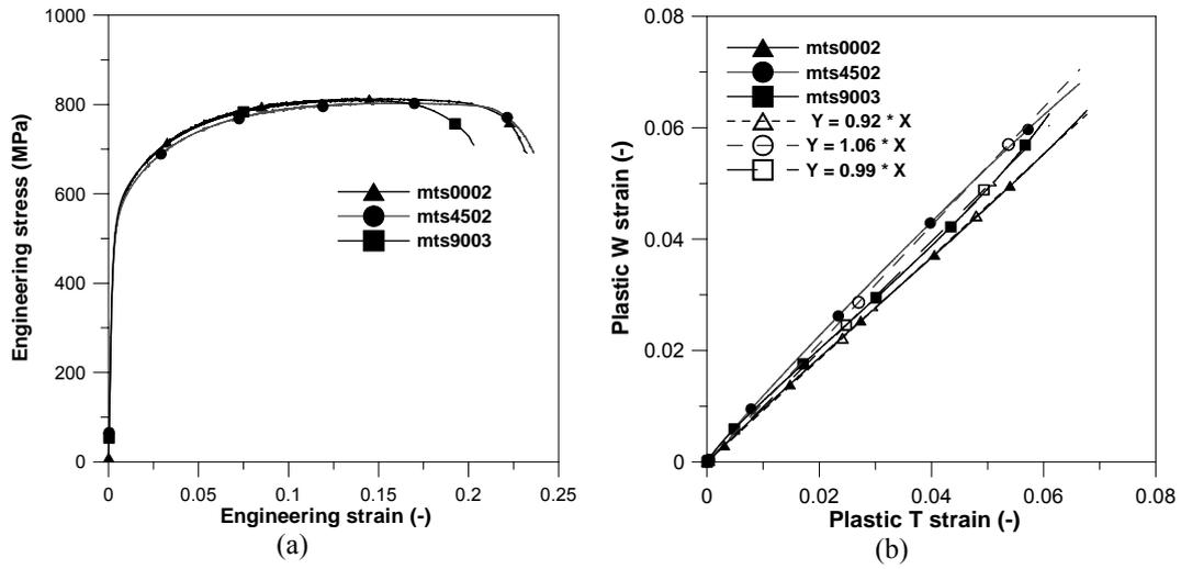
Fig. 8. Quasi-static tensile test results for one representative test in each direction of DP800, (a) engineering stress-strain curves, and (b) plots for determination of  $R$ -value
