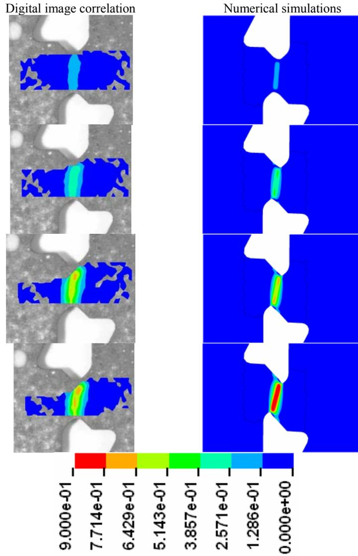
Fig. 16. Comparison of Green-Lagrange shear strain ( $E_{xy}$ ) plots at different deformation stages between digital image correlation (for mss02) and numerical simulations representing with the same colour scale
