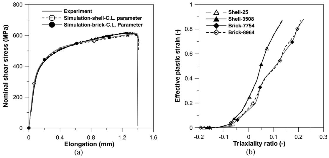
Fig. 15 (a) Experimental and numerical nominal shear stress vs. elongation curves after including failure parameter, and (b) comparison of plastic strain ( $\bar{\epsilon}$ ) vs. stress triaxiality ( $\sigma_m/\bar{\sigma}$ ) between shell and brick element simulations of shear test
