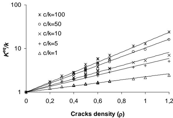
Figure 3. Increase of the equivalent permeability with cracks density for different values of  $c/k$
