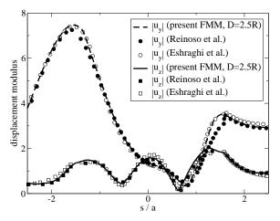
**Fig. 5** Scattering of SV waves by a semi-spherical canyon: horizontal and vertical computed displacement on line ABCDE (with points A, B, C, D, E defined on Fig. 3) plotted against normalized arc-length coordinate s/a along ABCDE ( $\theta=\pi/6$ ,  $k_{\rm S}a=0.75\pi$ )
