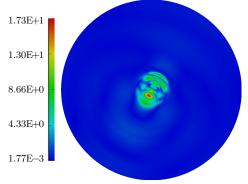
Fig. 10 Diffraction of an oblique incident SV plane wave by a semi-spherical basin: computed z component of displacement on basin surface and meshed part of free surface (normalized frequency  $k_{\rm S}a=2\pi$ )
