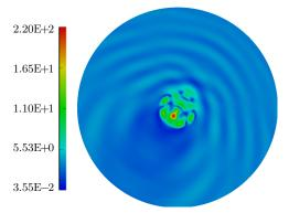
Fig. 8 Diffraction of an oblique incident SV plane wave by a semi-spherical basin: computed x component of displacement on basin surface and meshed part of free surface (normalized frequency  $k_{\rm S}a=2\pi$ )
