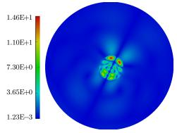
Fig. 9 Diffraction of an oblique incident SV plane wave by a semi-spherical basin: computed y component of displacement on basin surface and meshed part of free surface (normalized frequency  $k_{\rm S}a=2\pi$ )
