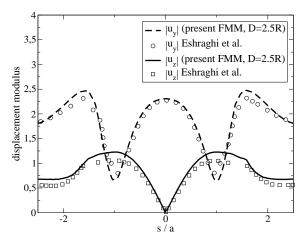
**Fig. 4** Scattering of SV waves by a semi-spherical canyon: horizontal and vertical computed displacement on line ABCDE (with points A, B, C, D, E defined on Fig. 3) plotted against normalized arc-length coordinate s/a along ABCDE ( $\theta=0,\ k_{\rm S}a=0.75\pi$ )
