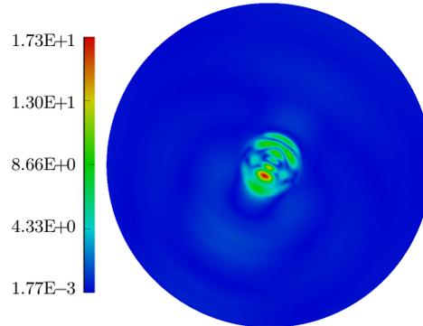
**Fig. 10** Diffraction of an oblique incident SV plane wave by a semi-spherical basin: computed  $z$  component of displacement on basin surface and meshed part of free surface (normalized frequency  $k_S a = 2\pi$ )
