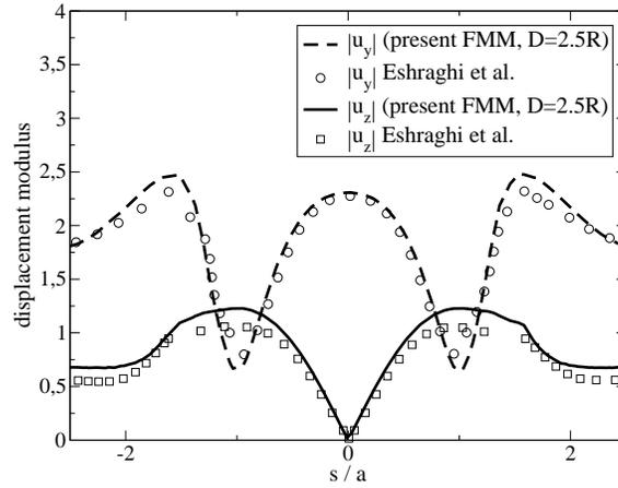
**Fig. 4** Scattering of SV waves by a semi-spherical canyon: horizontal and vertical computed displacement on line ABCDE (with points A, B, C, D, E defined on Fig. 3) plotted against normalized arc-length coordinate  $s/a$  along ABCDE ( $\theta = 0$ ,  $k_S a = 0.75\pi$ )
