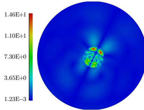
**Fig. 9** Diffraction of an oblique incident SV plane wave by a semi-spherical basin: computed  $y$  component of displacement on basin surface and meshed part of free surface (normalized frequency  $k_S a = 2\pi$ )
